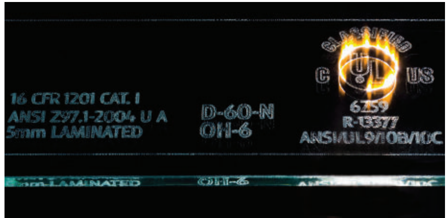
Figure 1. Laser marking with a CO 2 laser and an optimized scan head is performed on standard glassware ( opening image ) and architectural glass ( above ).
