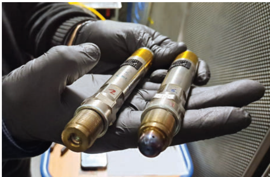
Figure 3. A close-up view of the type of laser spark plug used in the ignition experiments. A plug without a prechamber (left).
