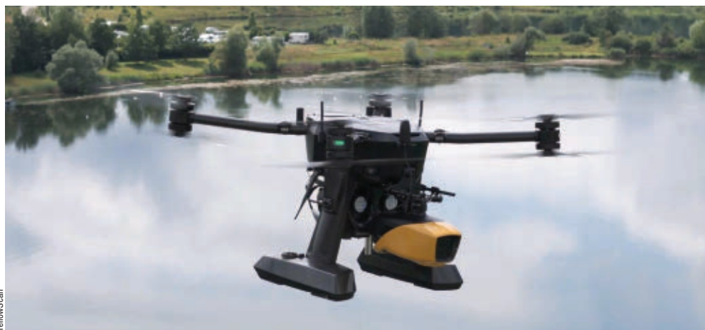
A drone carries YellowScan's bathymetric lidar system. The lidar system uses a green laser at 532 nm for underwater scanning.
