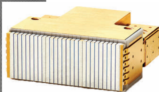
Figure 2. Advancements in facet passivation technology have increased the damage threshold of the facet to withstand ever-higher photon densities in laser diode architectures ( above ). Aluminum gallium arsenide (AlGaAs) is the semiconductor material in the laser structure. The crystalline layer adjacent to the AlGaAs layer is the high-damage-threshold (HDT) facet protection layer ( left ).
