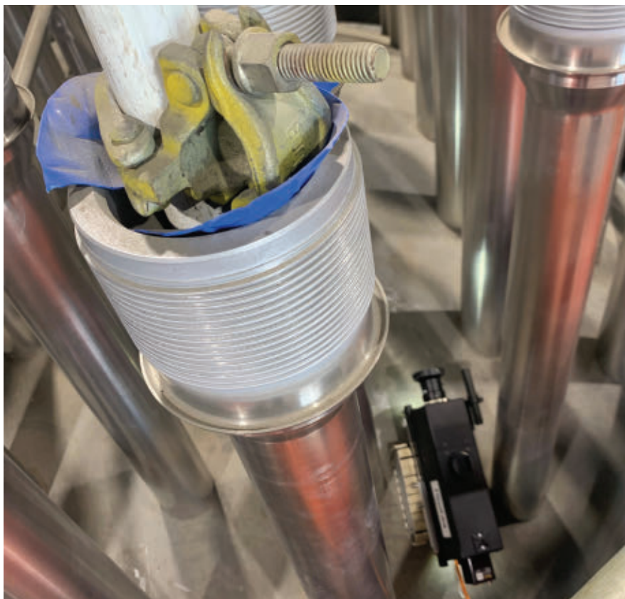
Hinalea's Model 4400, mounted to a 'magnetic crawler,' images a decommissioned nuclear reactor head ( left ). The hyperspectral camera is tested for its ability to detect pipe leaks by identifying the presence of boric acid corrosion ( above ).
