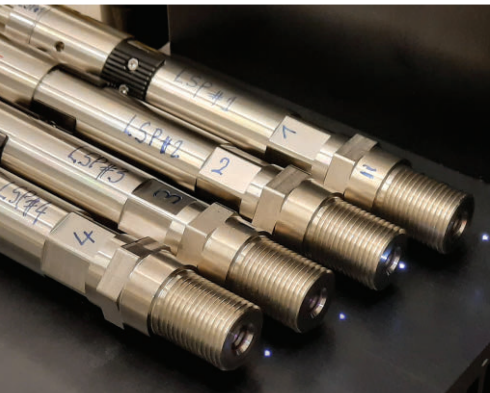
Figure 2. A set of four laser spark plugs during assembling and performance tests. The small sparks are laser plasmas, created due to air breakdown.
