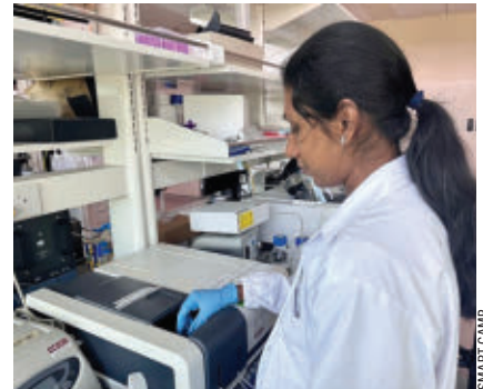
Shruthi Pandi Chelvam, a senior research engineer at the Singapore-MIT Alliance for Research and Technology Critical Analytics for Manufacturing Personalized-Medicine (SMART CAMP), uses an ultraviolet absorbance spectrometer to measure the absorbance spectra of cell culture samples.
