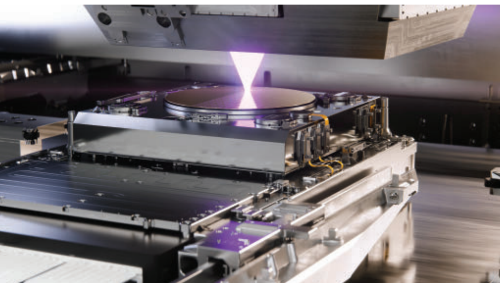
A manufactured wafer is exposed in a high-numerical aperture (NA) extreme-ultraviolet (EUV) system (impression) (left) .
