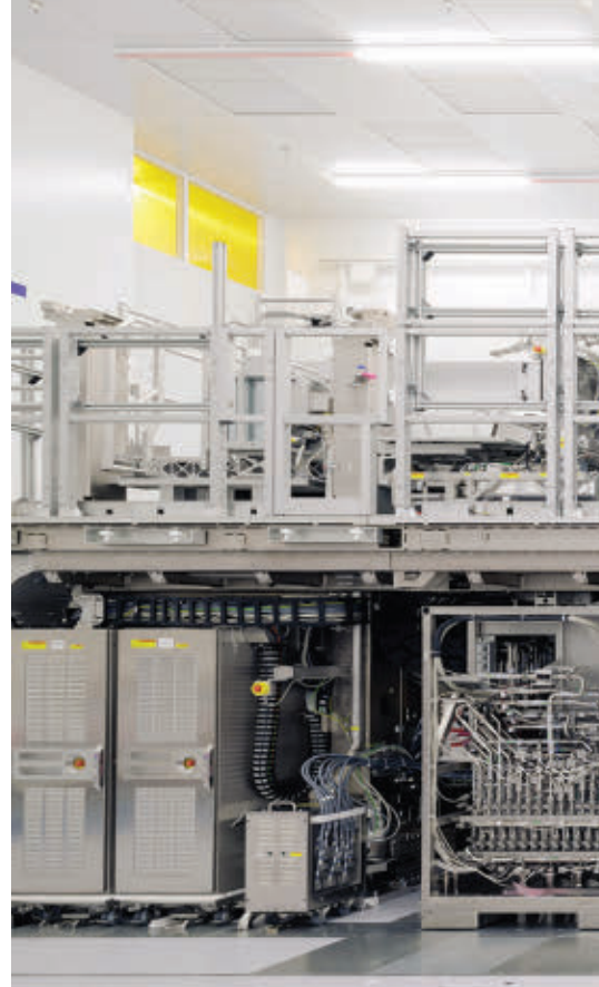
ASML's high-numerical aperture (NA) extreme-ultraviolet (EUV) system represents the chipmaking industry's gateway to the invaluable 13.5-nm wavelength.
