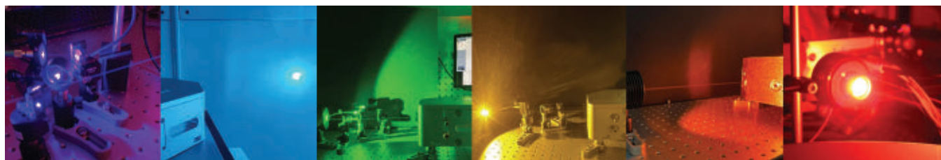
Figure 4. Uncorrected images of high-power single-mode laser output demonstrating the wavelength versatility of vertical-external-cavity surface-emitting lasers (VECSELs) ( above ). Atomic-based quantum technologies require a broad wavelength spectrum of high-power single-mode lasers. VECSELs address the requirement, emitting from the ultraviolet into the infrared.
