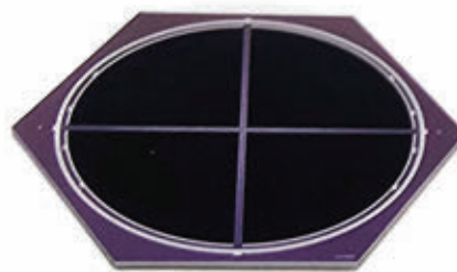
Figure 2. A black silicon four-quadrant detector chip ( above ) and a packaged component optimized for 1064 nm. In addition to defense applications, black silicon-based four-quadrant detectors are beneficial for other applications for which precise laser beam tracking or alignment is needed. The technology holds promise for medical imaging technologies and industrial process control. Black silicon nanostructures could also enable new capabilities in scientific instrumentation and analytical devices operating in the NIR.
