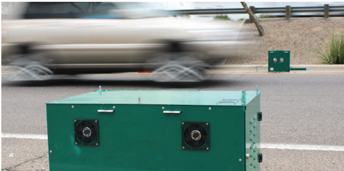
Opus Inspection Inc.'s remote sensing systems enable roadside emissions inspection in real time using fast-response photodiode arrays to measure vehicle emissions.
