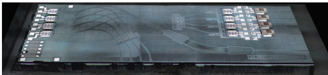
An interposer. Flat, combined electronic and photonic capabilities power the modern data center ( below ).
