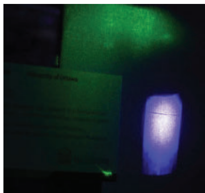
Researchers showed that a laser beam can sometimes act as a solid object and cast a shadow that is visible to the naked eye. The shadow appears as the horizontal line traversing the blue background.
