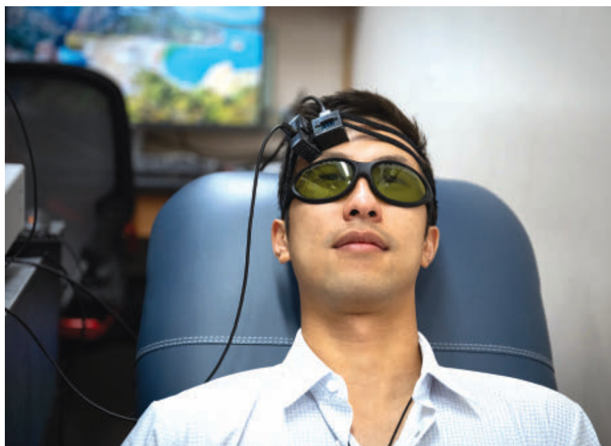
Researcher Yu Xi Huang, wearing the speckle contrast optical spectroscopy device, which can assess stroke risk.
