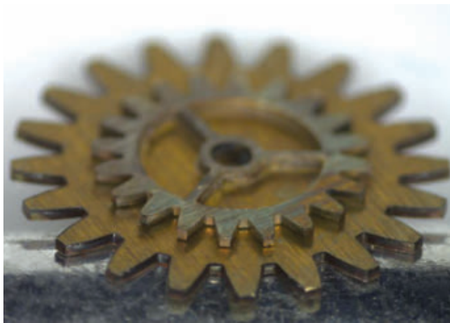
Figure 4. A demonstration of ultrashort-pulse (USP) laser processing shows cutting and welding of microscopic watch parts from brass ( top, right ) and an ablation of 3D shapes and surface texturing.
