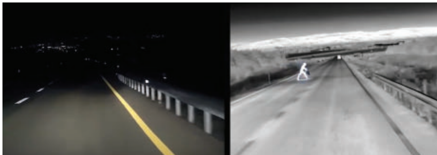
Nighttime detection with combined visible and thermal imaging. ADASKY's shutterless LWIR camera is designed to withstand harsh requirements: -40 to 85^{\circ}\text{C} .
