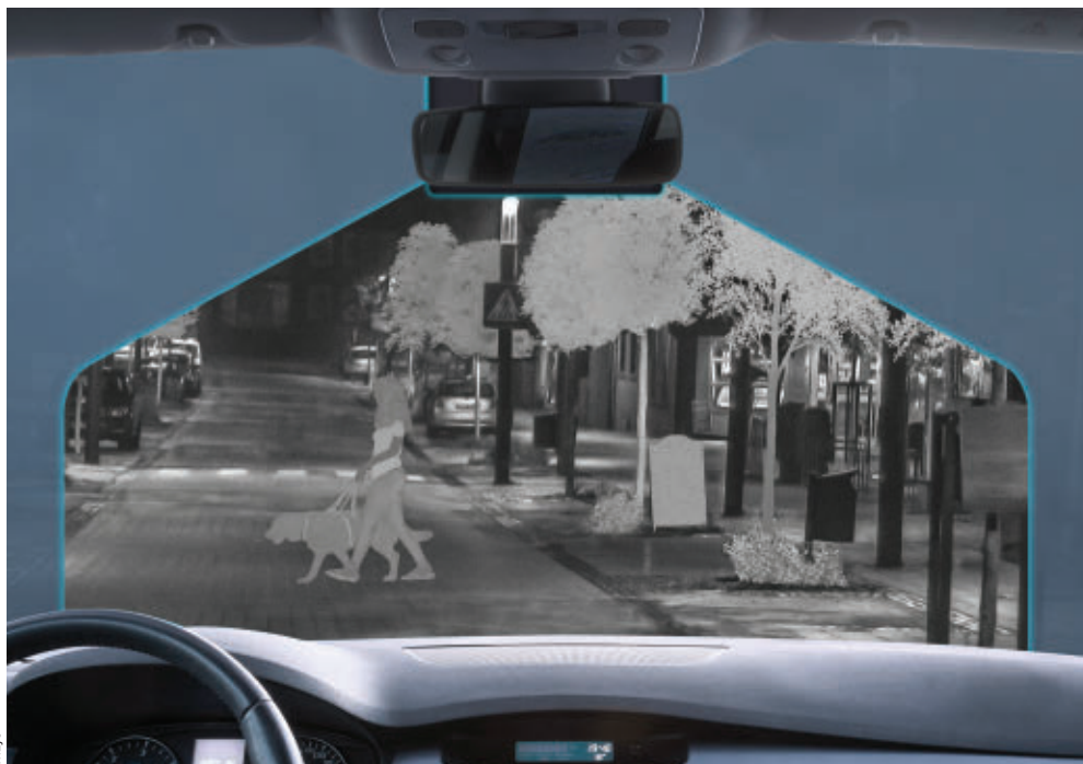
Windshield glass is opaque to LWIR light, which means that system integrators are unable to place many thermal cameras behind standard windshields. TriEye's SWIR technology can be placed behind windshields as well as headlights.
