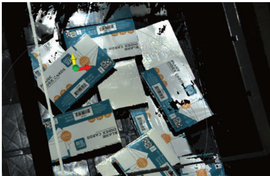
A 3D representation of random objects in a bin for robotic guidance.
