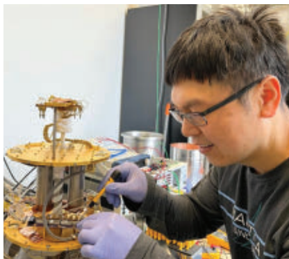
Fermilab scientist Si Xie mounts a superconducting nanowire single-photon detector inside a cryostat. Xie and his colleagues will use the detector to look for light created by dark matter particles.
