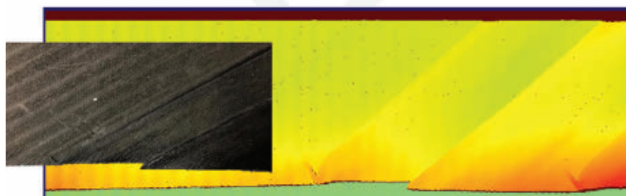
An image showing a defect in 3D using profilometry.
