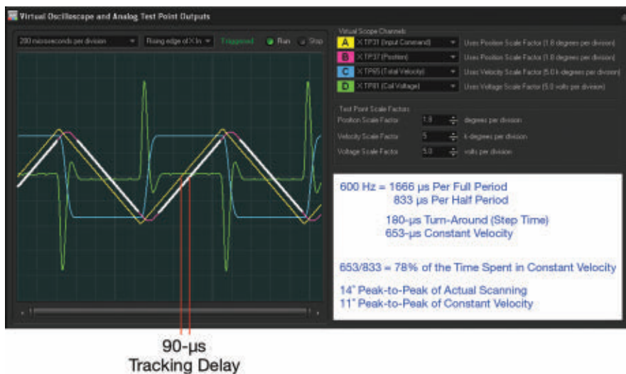
Figure 6. When the beam is traveling at constant velocity (blue), the position is highlighted (white). The velocity is constant, but there are short periods of time when the mirror must slow down, turn around, and speed up again. These areas (pink) are not highlighted and correspond with the scanner's step time.
