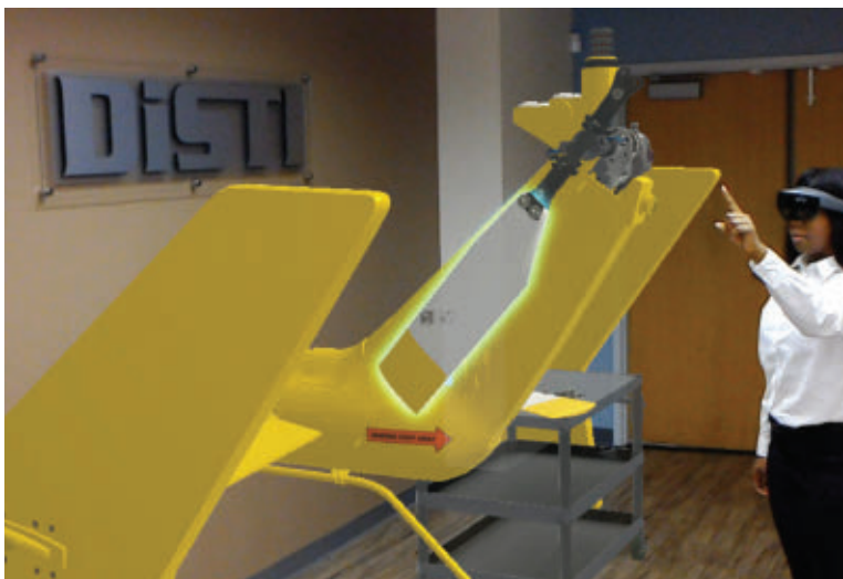
Merged reality, which combines the real and synthetic, is being used for maintenance training, in part because it allows collaborative training.
