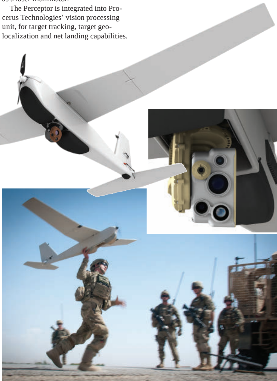
AeroVironment's Puma AE is equipped for land and maritime operations. Its gimbaled payload (inset) includes a stabilized IR camera and IR illuminator in one modular payload.
