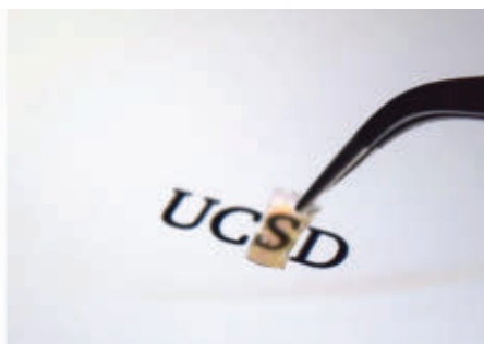
A near-perfect broadband absorber that’s thin, flexible and transparent in visible light.
