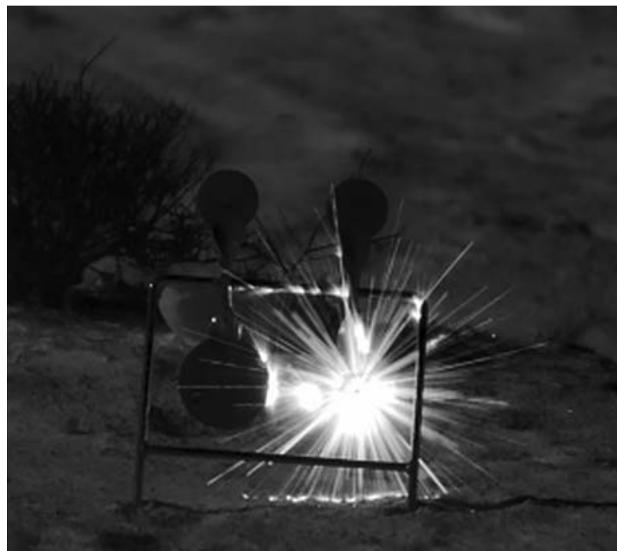
High-speed thermal camera image of .45 bullet hitting a steel plate.
