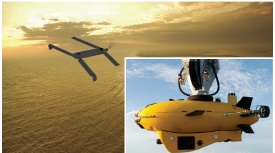
Lockheed Martin’s Vector UAV in flight. Last year, the Vector was canister-launched from the unmanned Martin submarine.
