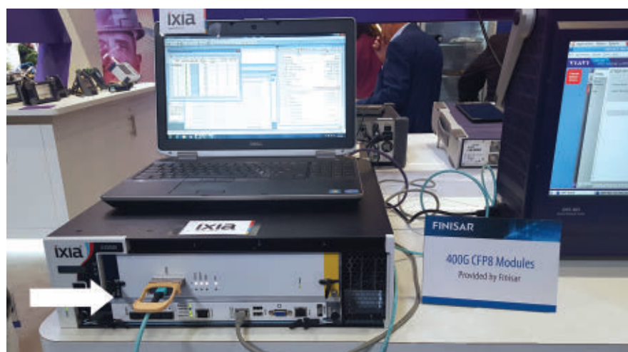
Demonstration of a pluggable 400G module, with four times the current commercially deployed connection speeds, interoperating with test equipment.
