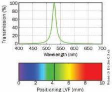
Spectral scan and relative scale available for linear variable bandpass filters.
