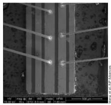
A scanning electron microscope image of the terahertz quantum cascade laser.
