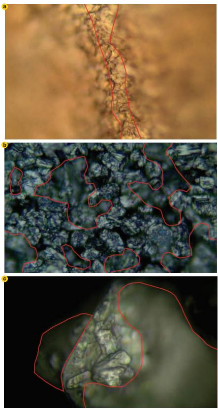
Figure 3. Optical images of (a) a tilted sample (graphene on a metal foil), (b) a rough sample (electrode from lithium ion battery) and (c) a sample with complicated surface geometry (a crystalline powder, I-cysteine).
