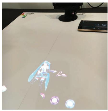
MEMS-based scanning technology enables tabletop projection. Smart projectors with integrated mobile operating systems could allow for interaction with the projected image.
