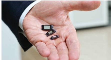
Manufacturing advances have resulted in smaller MEMS feature sizes, which in turn means that projection display chips have gotten smaller.
