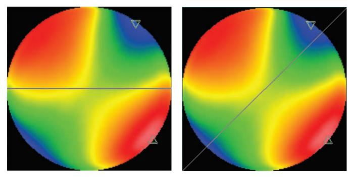
**Figure 1.** Interferogram with sample 2D traces. (Left) Horizontal:  $PV = 0.790\lambda$ , rms = 0.195 $\lambda$ . (**Right**) Diagonal:  $PV = 1.841\lambda$ , rms = 0.546 $\lambda$ . (PV = peak-to-valley, rms = root mean square)
