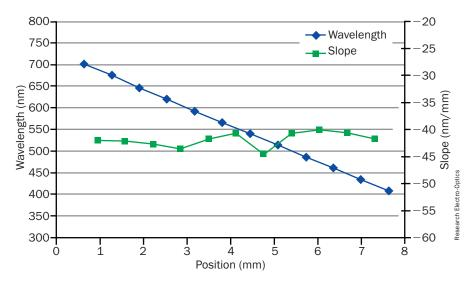
Typical linear variable filter center wavelength and slope vs. filter position.
