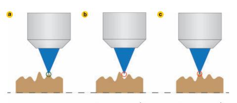
**Figure 1.** Change in focus of Raman light as sample is scanned underneath the objective: (a) Sample in focus, (b) focused above sample and (c) focused into the sample. In all cases, the sample volume probed and the Raman intensity will vary.
