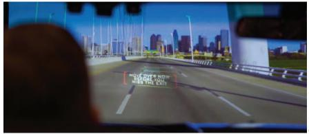
MEMS projection technology powers high-brightness and interactive head-up displays to enhance driving.
