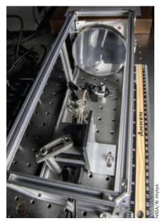
This laboratory breadboard is used to test a conceptual telescope for use on CubeSat missions.
