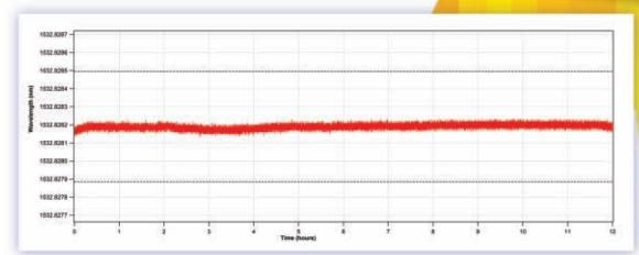
Long-term wavelength measurement data of a DFB laser locked to an absorption line of acetylene. The specified accuracy is given by the dashed lines.
