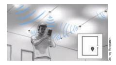
Conceptual illustration of EnLighting, an indoor visible light communications system.
