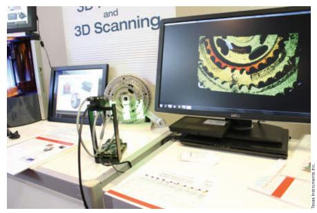
A MEMS digital micromirror device, camera and other peripherals enables 3D scanning through the use of structured light.
