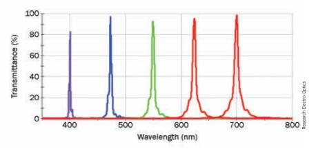
Linear variable filter design spectra vs. wavelength indicating change of bandwidth.
