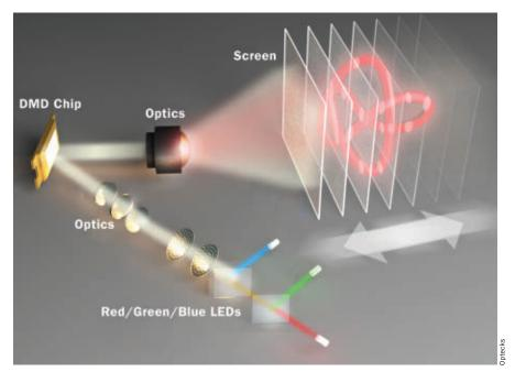
MEMS-technology can create 3D displays by maintaining image quality over several centimeters in depth.
