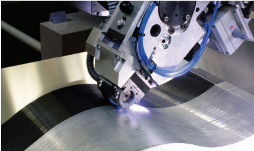
Lightweight components are manufactured using a new method: combining fiber-reinforced tapes with laser-induced heating. Courtesy of Fraunhofer Institute for Production Technology.
