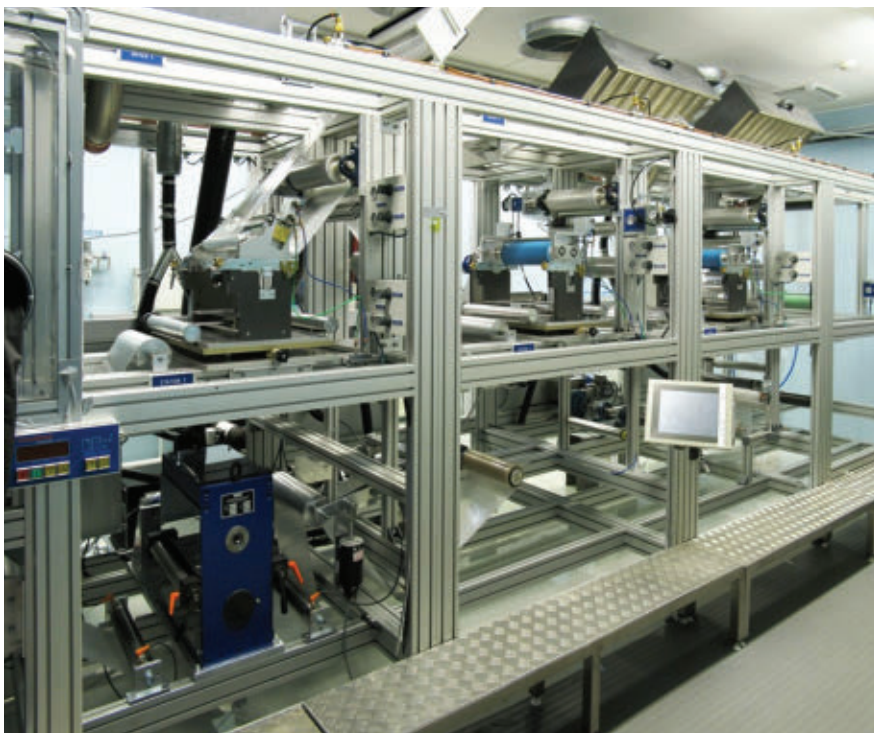
Figure 1. Shown is a pilot printing machine for printed electronics. Images courtesy of VTT Technical Research Centre of Finland, Printed Functional Solutions.
