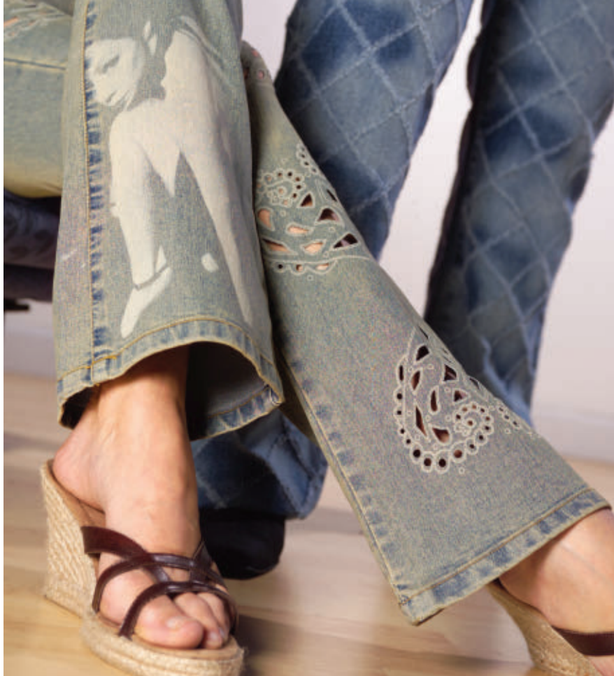
Figure 4. Sealed carbon dioxide lasers are now widely used for engraving and marking of a wide range of organic materials, with possibly no application more eye-catching than the production of images, cutouts and fake 3-D effects on high-end denim jeans. Courtesy of Coherent Inc.
