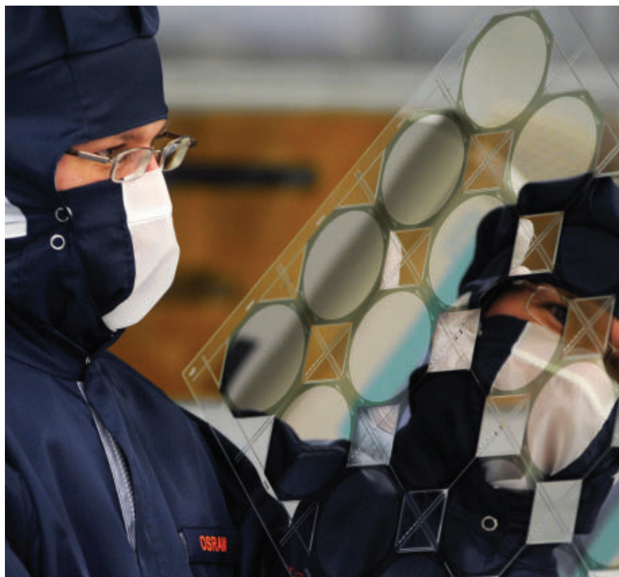
An employee of Osram Opto Semiconductors checks the coated OLED panels for regularity. The focus here is on purity as well as the displacement of different coatings. Images courtesy of Osram Opto Semiconductors.
