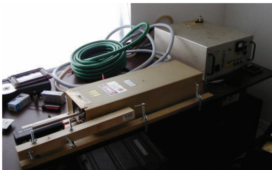
Shown is a Uniphase HeNe laser, the Lexel 88 argon-ion, and its power supply. Courtesy of photographer Gregory Maxwell.
