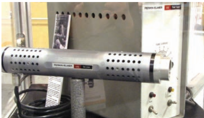
Perkin-Elmer and Spectra Physics collaborated to make the early HeNe laser (left) in 1963. Perkin-Elmer modified the design to create the model shown on the right in 1966.
