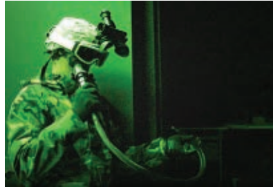
Schott's NightViper optical scope, introduced by the company's Fiber Optics Defense Division in 2008, allows soldiers on night operations to see what's around corners, under doors, in vehicles or through holes in buildings before entering. NightViper, a flexible wound fiber optic bundle 2 to 6 ft long, attaches to standard 18-mm night-vision goggles. (Photo courtesy of Schott)
