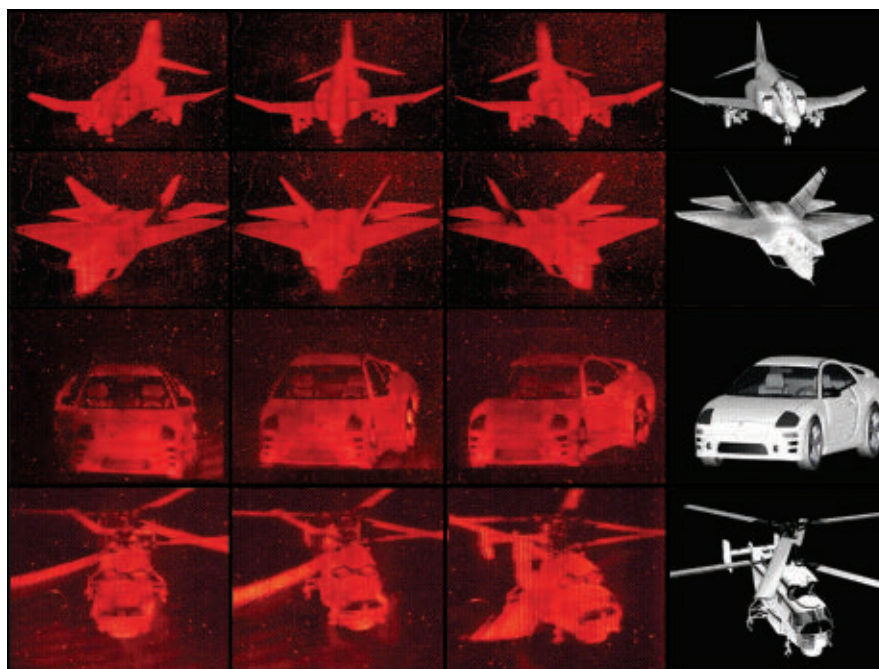
Rewritable holograms, such as these, could allow three-dimensional rendering of battlefields and other military command-and-control applications. Courtesy of Nasser Peyghambarian group, University of Arizona.
