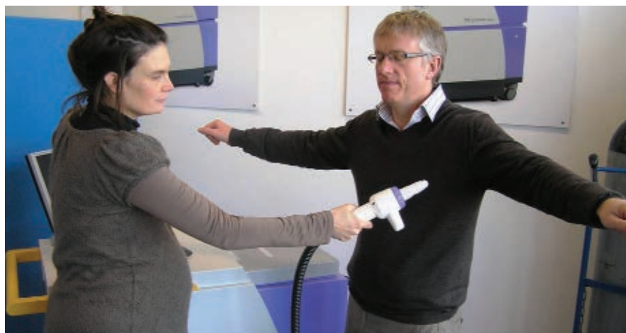
TeraView offers people screening capabilities using terahertz light. Courtesy of TeraView.
