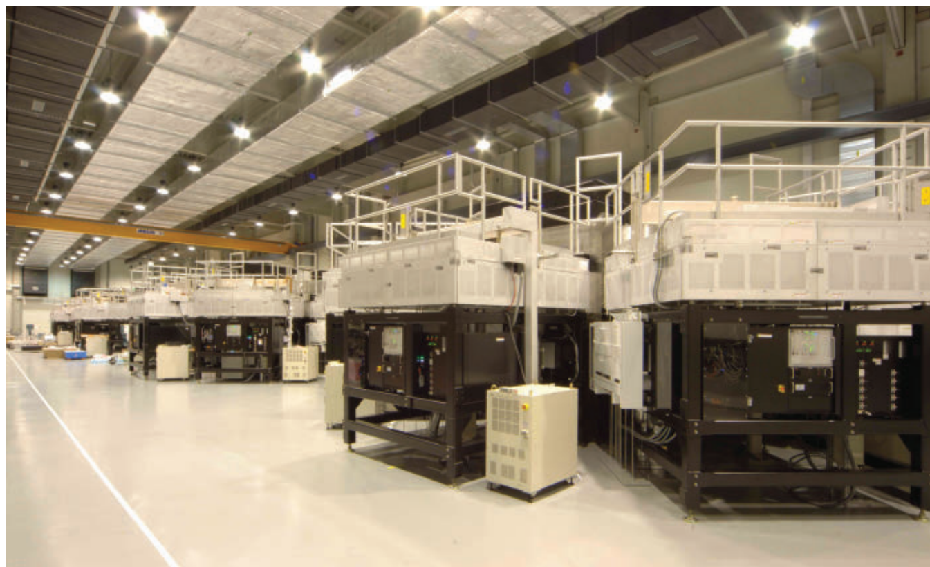
Sunfilm's production facility manufactures tandem junction thin-film solar modules in Großröhrsdorf, Germany. The plasma-enhanced chemical vapor deposition system is important for depositing critical light-absorbing silicon layers on 5.7-m 2 glass substrates, with the quality of the coating being checked by optical metrology systems. Courtesy of Business Wire.
