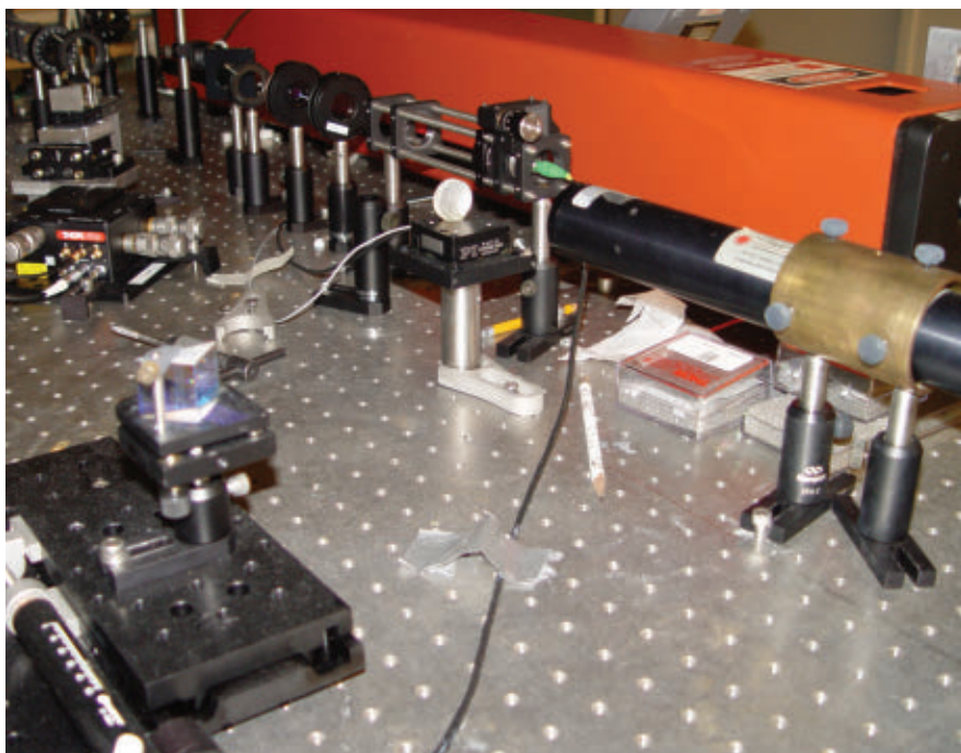
This is the experimental setup used to determine propagation delays of photons traversing dielectric stack structures. Courtesy of the Joint Quantum Institute.
