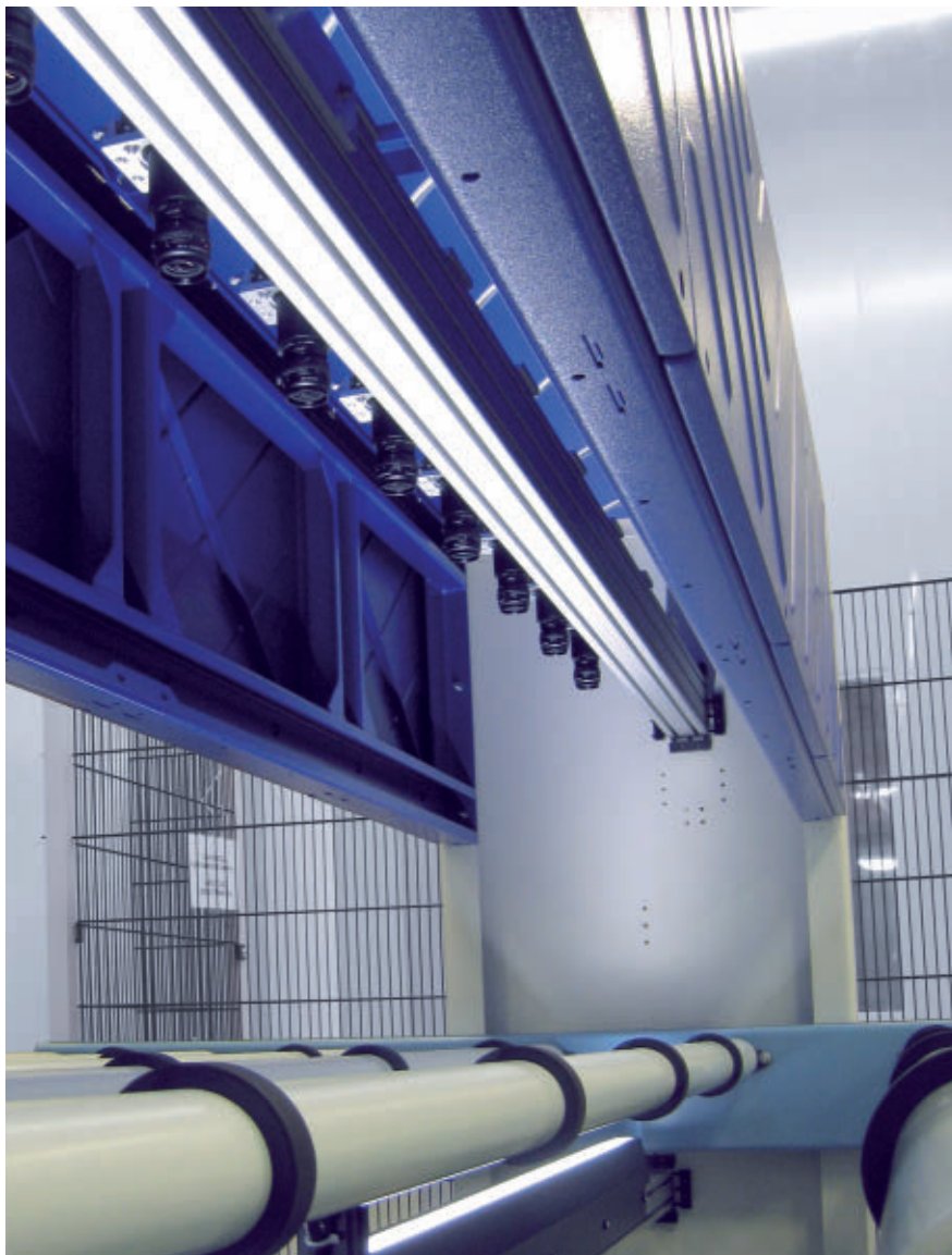
Pictured is Basler's imaging system, first developed for liquid crystal display manufacturing and now integrated into a solar cell production line that can process 5.7-m 2 glass substrates. The system helps improve efficiency and reduces the cost of solar module manufacturing.
