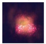
This photo shows a microscopic image of an electrically conducting polymer film that was pumped by a pulse of green light from a conventional laser, exciting tiny cavities within the film to produce redcolored "random laser" light. Photos by Randy Polson, Department of Physics and Astronomy, University of Utah.
