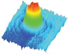
A 3-D rendering of a thermal map of the sphere pressed into the surface with a force of 3.1 N highlights that the cooler contact areas in the center (red) occur where the heat loss from the surface is greater.
