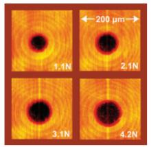
Thermal images of the contact between the sphere and the flat surface reveal that, as the sphere is pressed with greater force (increasing from upper left to lower right), the surface contact area increases. Images courtesy of Oliver Wright of Hokkaido University.
