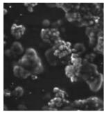
A film of the polymer DOO-PPV, as seen through a microscope, shows clumps of undissolved polymer within the darker, dissolved material. Such irregularities are believed to create the tiny cavities that act as built-in mirrorlike resonators for random lasers.
