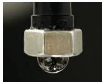
A close-up of the 6-mm-diameter ceramic ball attached to the mechanical arm.
