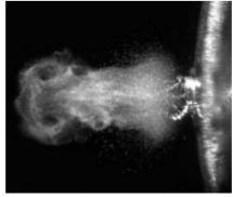
Shown is a plume captured 24 µs after a 2.94-µm laser shot struck glycerol. By studying how such plumes evolve over time, researchers can improve how much material is ionized and thus becomes suitable for mass spectrometry. Courtesy of Kermit K. Murray, Louisiana State University.
