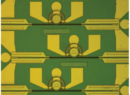
A hybrid silicon ring laser, like the three shown here, could be used as an on-chip light source in future photonic circuits. The 12.5-µm-radius rings in the image consist of a III-V compound semiconductor. Waveguides – the black lines running below the rings – connect two integrated photodetectors. Courtesy of Di Liang, University of California, Santa Barbara.
