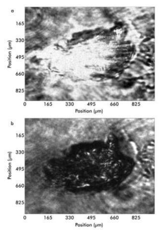
Shown are shadowgraphic images of a 100-µm-thick glass target shot with a high-energy laser both without (a) and with (b) the use of an optical Kerr gate. Reprinted with permission of *Applied Physics Letters*.
