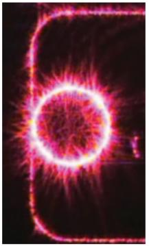
Shown here is a U-shape waveguide that glows because the light is tuned to the resonant frequency of the ring in the center. In practice, this structure would act as a modulator by injecting charge into the silicon, thereby tuning the ring's frequency as needed to allow light to pass, or to stop it from doing so. Courtesy of Hewlett-Packard.
