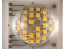
The multichip XLamp MPL EasyWhite LED manufactured by Cree Inc. is suitable for directional lighting applications, including PAR- or BR-style
