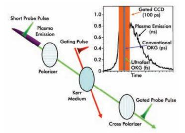
Using an optical Kerr gate is the key to ultrafast imaging of laser-induced plasma, according to researchers at Rutherford Appleton Laboratory and at Imperial College London. The CCD used for imaging is placed behind crossed polarizers; aiming intense gating pulses at the nonlinear Kerr medium alternates its birefringent state, permitting a quick shuttering effect. Courtesy of Dan Symes, Rutherford Appleton Laboratory.
