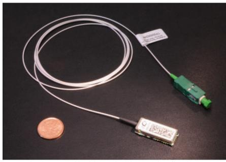
Compact PLC-based transceiver module includes a wavelength division multiplexing filter, a laser, multiple detectors, an amplifier and other subcomponents all integrated onto the PLC chip.
