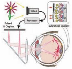
A diagram of the photovoltaic retinal prosthetic system includes a video camera, an image processor, a pulsed infrared microdisplay inside video goggles and a subretinal photovoltaic array.
