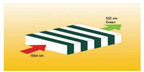
HC Photonics Corp. gets the green light needed for picoprojectors from frequency-doubling an infrared input. Courtesy of HC Photonics.
