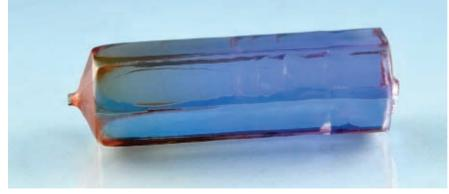
An improved crystal-growing method allows Castech Crystals Inc. to manufacture larger  $Nd:YVO_4$  crystals. Courtesy of Castech.
