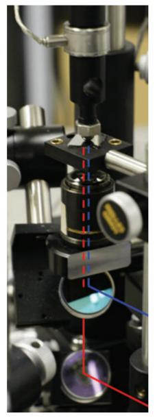
The mechanical arm presses the ceramic ball down onto the chromium surface. The red line is the excitation beam or pump laser, and the blue line is the detection beam or probe.
