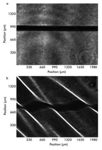
Not all materials are equal candidates for use as optical Kerr gates. Zinc oxide works fairly well (a), although it absorbs pulse probes around 400 nm. Leadbismuth glass (b) produced striations in the image, which excludes it for future consideration. Reprinted with permission of *Applied Physics Letters*.
