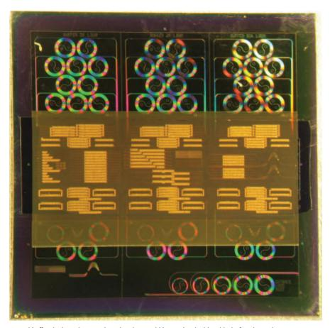
Optical buffers built in silicon, such as this chip, could be used as building blocks for silicon photonic circuits. The rings seen here function as long delay lines. Courtesy of John Bowers, University of California, Santa Barbara.
