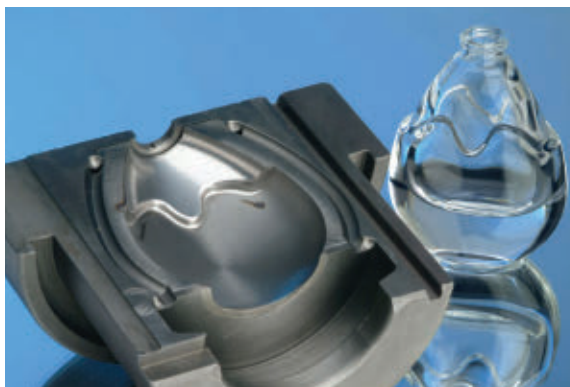
Free-form surfaces such as this mold require high-quality polishing to ensure seamless manufacturing and good surface quality of the mass product. To date, this has been a manual job, but now lasers can help.
