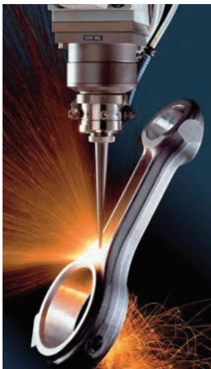
Above, the lines around the edge of the bright blue solar cell are made by a laser. At right, a laser drills a hole in a connecting rod. The hole allows lubricant to flow to the contact surface. Courtesy of Trumpf.
