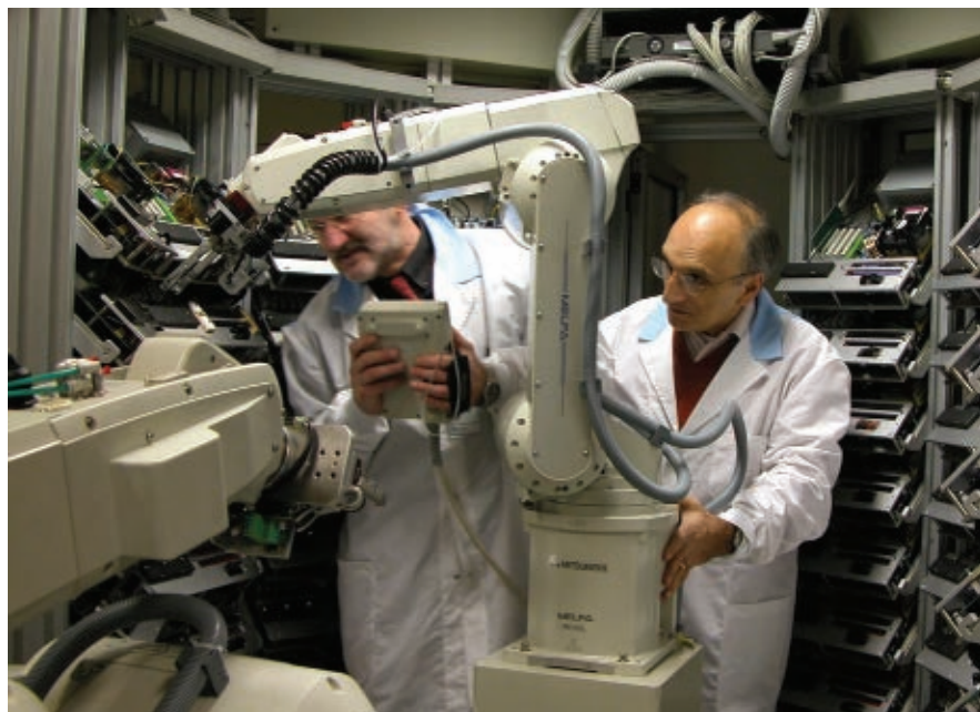
To avoid collisions while operating in tight confines, robots increasingly will use vision guidance, as are the ones shown here, which are involved in fully automated memory chip testing. Courtesy of ImagingLabs.
