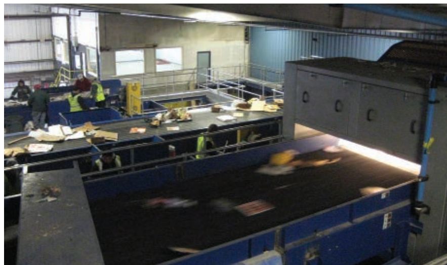
Vision sensors won't take out the trash, but they are helping to sort it with recycling systems such as this short-wavelength infrared-based solution. Courtesy of Eagle Vizion.
