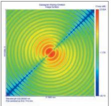
BSP supports full-vector field propagation. This decibel-scale plot shows the Z-component of the focal plane intensity of a Ritchey-Chrétien telescope for linearly polarized light.
