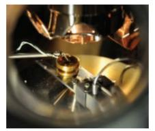
Use of an ionic liquid enabled researchers to perform spectroscopy of electrochemically generated species during a reaction in an ultrahigh vacuum. X-rays produce photoelectrons from the electronic core of analytes placed in the ionic liquid. Courtesy of Peter Licence, University of Nottingham.
