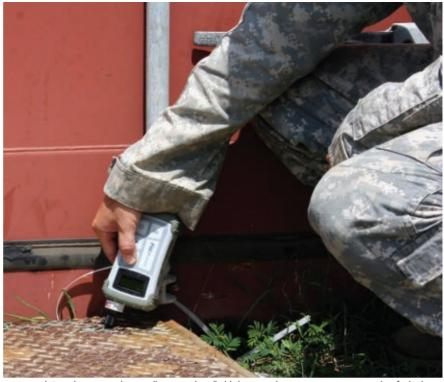
A National Guardsman samples a spill, using a handheld device and Raman spectroscopy to identify the liquid. Courtesy of ICx Technologies.
