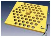
This schematic graph shows the system of a nanorod coupled with the cavity of a photonic crystal slab. Notice that the system axis Z is perpendicular to the slab (X-Y plane) in the figure. Images courtesy of Duke University.
