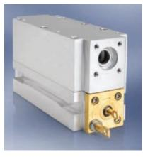
of output power and the Genesis 532-500 S models, >0.5 W. Both are aircooled, available in OEM packaging and can be directly modulated. Based on proprietary optically pumped semiconductor laser technology, they are scalable in wavelength and output power. Linewidth is <30 GHz FWHM, pointing stability is <10 µrad/°C, polarization ratio is >100:1, horizontal, and operating diode current is <10 A. Coherent tech.sales@coherent.com
