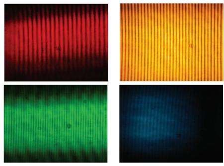
A frequency comb with teeth that can be seen is now possible, thanks to new laser technology. Showing the entire comb would comprise 1500 such photos. Courtesy of Scott Diddams, NIST, and Albrecht Bartels, Gigaoptics GmbH.
