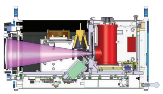
Radiation is focused by the objective lens onto an LN2-cooled detector. The path to the detector is interrupted by a reflective chopper wheel (shown in green), which alternately exposes the detector to the incident radiation and to the radiation from the internal blackbody source (shown in orange).
