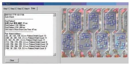
New software algorithms are being developed to speed up LCD inspection without sacrificing manufacturing speed. Courtesy of Chern-Sheng Lin, Feng Chia University, Taiwan.
