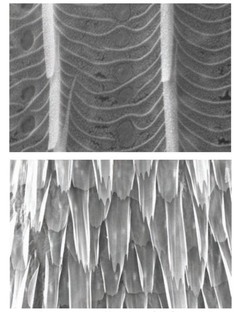
Two scanning electron microscope images reveal the external structure of a butterfly wing coated with chalcogenide glass. The removal of the wing by submersion in orthophosphoric acid allows the conformal coating and chitinous coating to separate from the wing, resulting in a free-standing replica.
