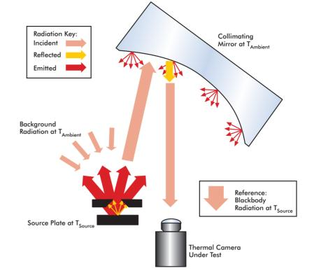
The cooler background radiation does not compensate entirely for the imperfect emissivity of the target, and the radiation from the ambient temperature mirror does not fully compensate for its imperfect reflectivity. The result is that the radiation presented to the camera under test appears to have originated from a blackbody at a temperature less than the physical temperature of the source.
