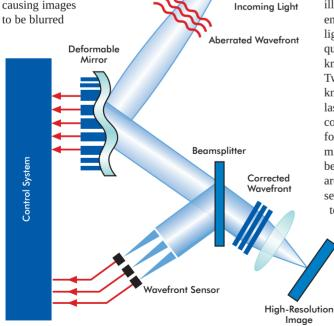
Figure 1. There are three main components of an adaptive optics system: a sensor to measure wavefront aberrations, a deformable mirror that can correct for the aberration, and a control system that takes measurements from the sensor and calculates the necessary movement of the mirror. Adapted from Professor Claire Max, director of the Center for Adaptive Optics, University of California, Santa Cruz.
