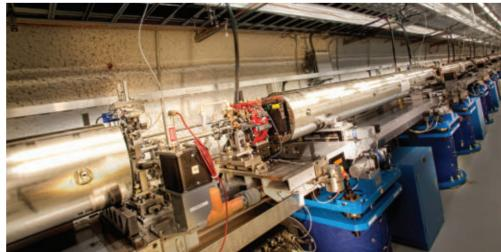
Thirty-three Linac Coherent Light Source undulator magnets create intense x-ray laser light from a pulse of electrons traveling 99.9999999 percent the speed of light. Courtesy of Brad Plummer, SLAC.
