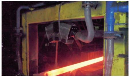
Hot steel glows visibly as it emerges from a push bench, making automated machine inspection of the surface difficult. Images courtesy of José Angel Gutierrez, Robotiker-Tecnalia.
