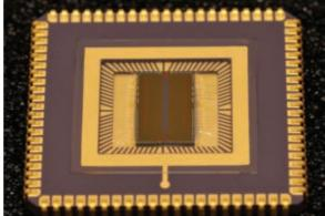
The innovative CMOS image sensor can distinguish color and is much more light-sensitive than conventional sensors. Image Fraunhofer IMS.
