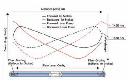
This schematic depicts an ultralong Raman fiber laser design and optical power distribution. Pumping at 1450 nm generates laser radiation at 1550 nm. Reprinted with permission from Turitsyn et al, *Physical Review Letters*, 103, 133901 (2009). ©American Physical Society 2009.
