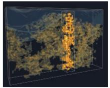
This 3-D electron tomography image of the inside of a polymer-metal oxide solar cell shows the metal oxide network (yellow) in the polymer phase (transparent) below an aluminum top electrode (gray). Most zinc oxide is interconnected and makes contact with the aluminum electrode.
