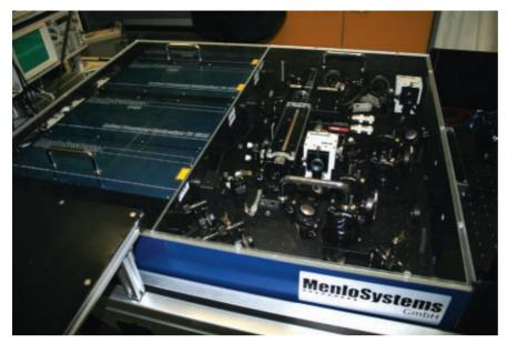
Shown is a transportable femtosecond comb laser that is used to measure the frequency of a stable laser source. The mechanism directly converts optical frequencies to low-frequency signals that can be electronically counted. Components include an erbium-doped fiber laser that produces a frequency comb operating at a range of 500 nm to 2.1 µm, a high-stability oscillator and a GPS-disciplined Rapco 2804AR rubidium oscillator. Courtesy of National Physical Laboratory.
