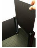
The Kentek table guard barrier system is highly configurable and can be fitted to any standard optical bench or to a customized layout, with options suitable for both imperial and metric optical tables. Its panels are composed of a propristem or acrufic
