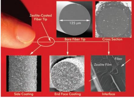
Zeolite's subnanometer-size pores trap molecules, enabling detection of explosives via an optical fiber. Courtesy of Hai Xiao, Missouri University of Science and Technology.
