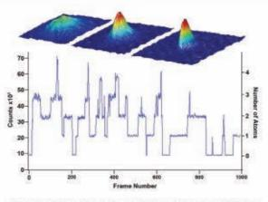
Top image: Surface plots of the transition from a thermail gas (laft) to a Bose-Einstein condensate. The sharp, bimodal peak in the right figure is a signature of a BEC.
