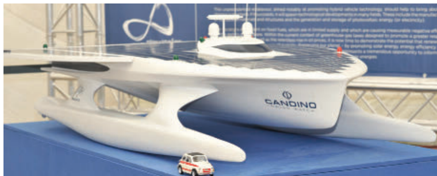
The PlanetSolar catamaran will have 470 sq m of solar cells on deck to power it around the world next year.
