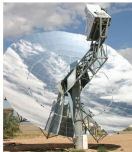
Each 11.6-m dish of the Sun Catcher is made up of 40 mirror facets, which are manufactured on automotive-type assembly lines.
