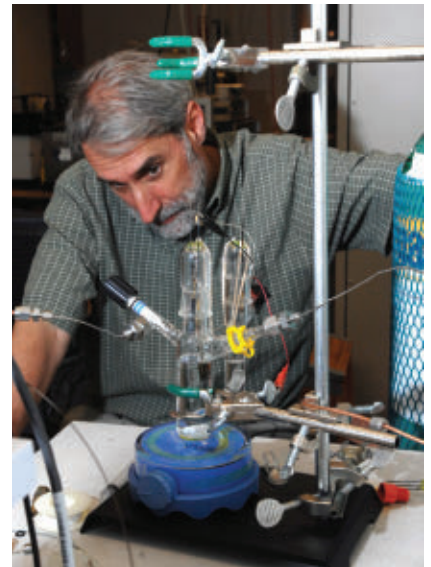
Daniel G. Nocera’s group at MIT uses the sun’s energy to split hydrogen and oxygen from any kind of water, using a cheap metal alloy as a catalyst. Photo by Donna Coveney, MIT.
