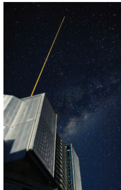
A laser guide star is generated by high-power laser radiation sent to the 90-km-high sodium layer in the atmosphere. Fluorescence emission generated there helps to compensate for optical aberrations caused by atmospheric turbulences.
