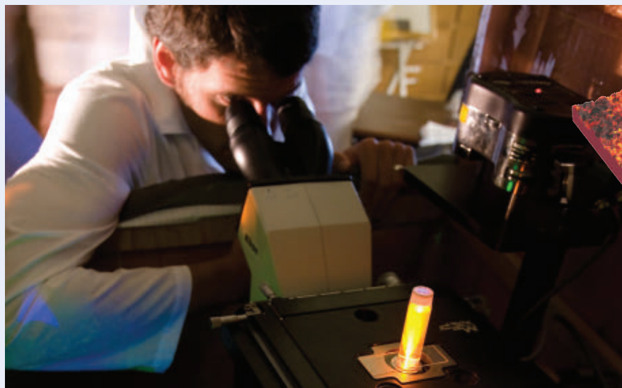
University of Washington doctoral chemistry student Obadiah Reid aligns the laser in a dual optical/atomic force microscope prior to performing photoconductive atomic force microscopy on nanostructured polymer solar cells.
