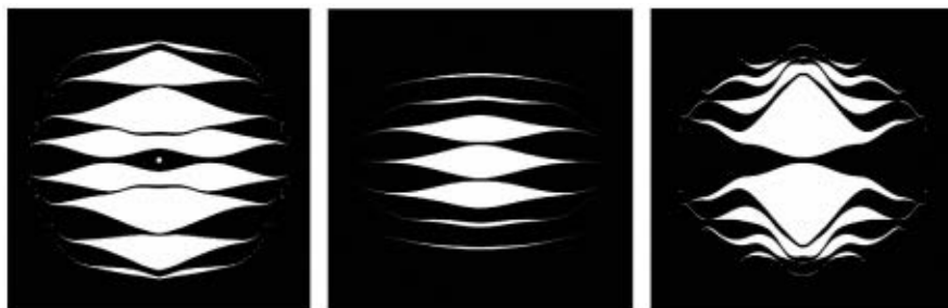
The Jet Propulsion Laboratory at the California Institute of Technology is investigating several internal coronagraph designs for the Terrestrial Planet Finder, including these possible binary mask shapes. Sample masks of this type have been fabricated using deep reactive ion etching of a 400-m-thick silicon-on-insulator wafer.
