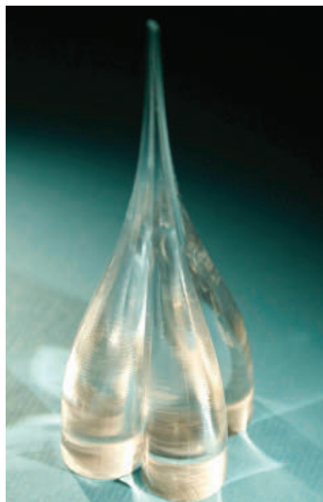
Figure 1. The Gemini fiber integrates ease of splicing and contacting with the concept of multicore fiber sensing. Photos courtesy of Acreo AB.
