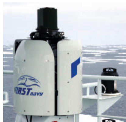
A thermal imager installed on the Polarstern's crow's nest at a height of approximately 28 m scans the ocean for surfacing whales. The sensor head (green) sits on a highly stabilized platform (white basis) and rotates at 5 rps. Courtesy of Lars Kindermann, Alfred Wegener Institute.
