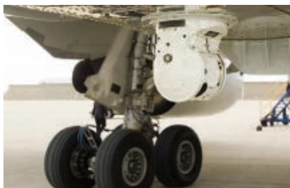
An element of the JetEye airliner IR missile protection system, the laser point-and-track "jam head" is fitted to the underbelly of a plane.
