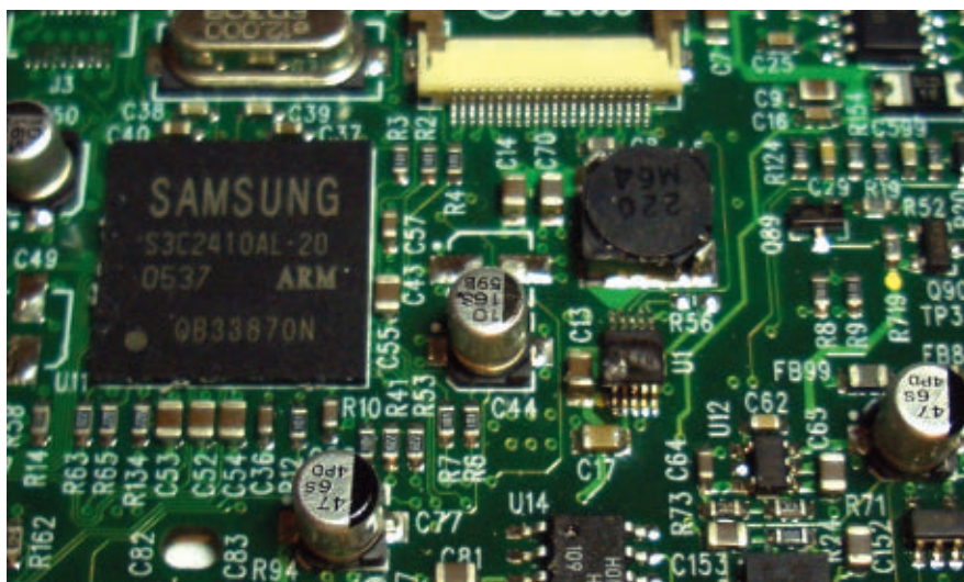
Portable microscopes are used for circuit board inspection, as seen here using 20× magnification. Image courtesy of Celestron.
