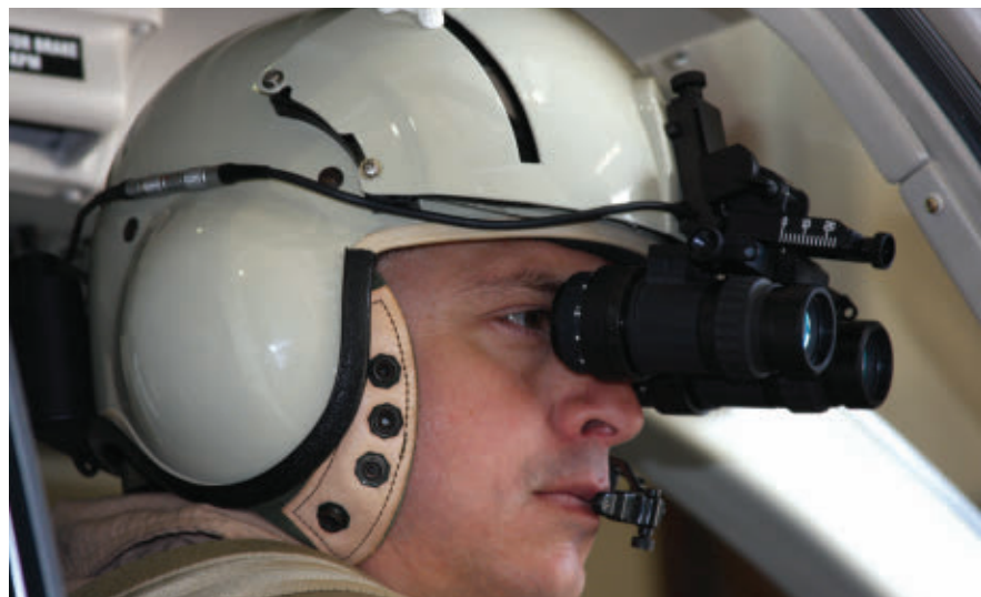
Shown is a pilot looking through the NVAG-6 goggles. Inside an aircraft, the pilot must shift his eyes below the goggles to see the instrument panel because the binoculars allow visibility only in the near-infrared spectrum. Courtesy of Nivisys Industries.
