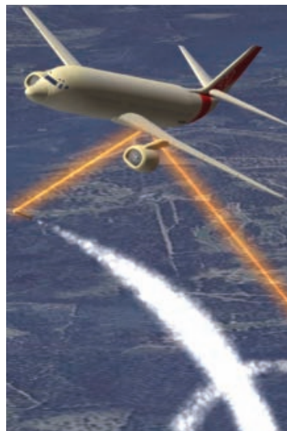
An artist's concept of a shoulder-fired missile being defeated by a laser-based IR countermeasure system on an airplane. Photos courtesy of BAE Systems.
