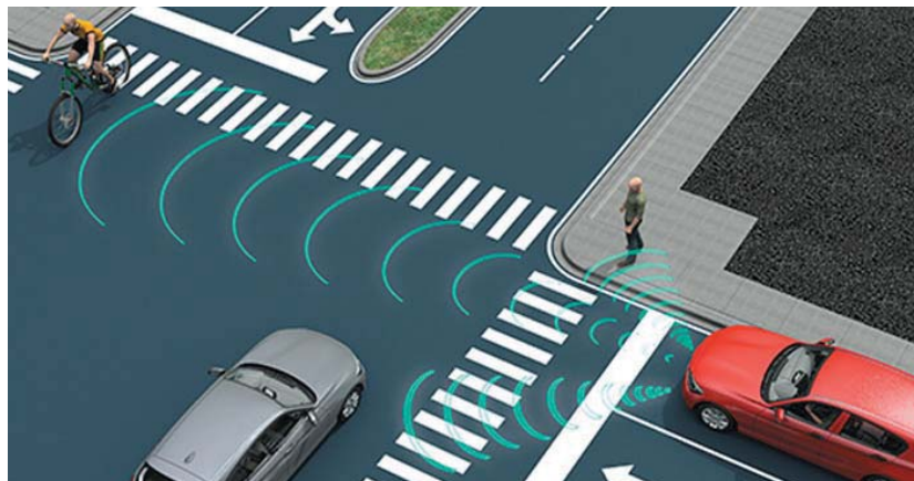
1. ADAS-equipped vehicles rely on fusion of sensor data from radars, LiDAR, and camera-based systems to create a 360-deg. field of target detection. (Courtesy of Xilinx)
