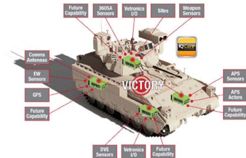
2. In this example of an open systems platform architecture, a single, unmodified eight-slot chassis design provides all required functionality of the platform with different plug-in module payloads.
