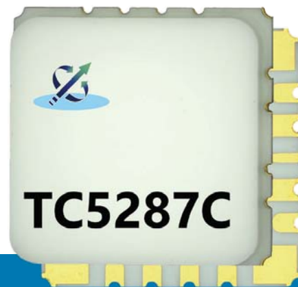
TC5287C & TC5285C 26.5-31.5GHz 3W High Linearity GaAs PA MMICs
