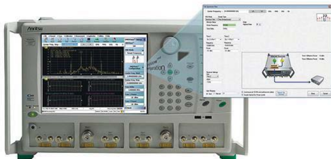
6. The VectorStar line of VNAs was greatly enhanced by the new IMD-View software for IMD measurements. (Photo courtesy of Anritsu Corp.)
