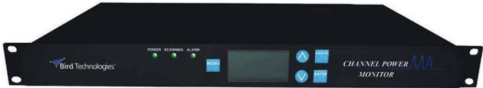
1. The model 3141 Channel Power Monitor occupies a single (1U) standard rack space. It features an integrated Web server with SNMP-based messaging, and accommodates up to 16 power sensor inputs.
