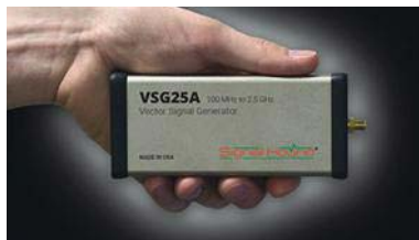
5. For signals through 2.5 GHz, the model VSG25A vector signal generator is truly a handful. (Photo courtesy of Signal Hound)
