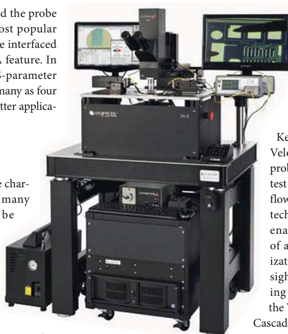
This adaptive architecture technology enables users to configure probe systems to meet specific application requirements. (Photo courtesy of SemiProbe)
