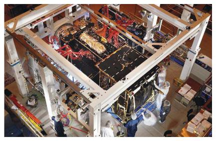
The SBIRS GEO-2 satellite undergoes baseline integration system testing. (Image courtesy of Lockheed Martin)
