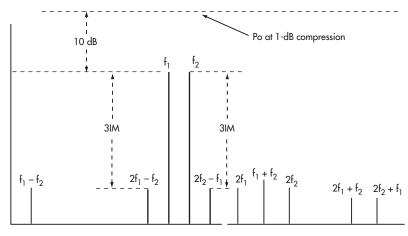
2. Duplex modulation techniques have a higher-power transmission band and a lowerpower reception band. Unfortunately, intermodulation-distortion products can appear in the reception band of the device, impairing signal reception.
