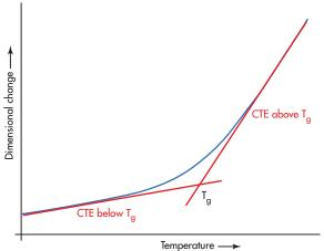
3. Maintaining consistent coefficient of thermal expansion (CTE) with temperature is beneficial for circuit materials for PAs and LNAs.
