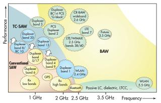
SAW and BAW filter technologies generally perform with high Qs and low insertion loss compared to other filter technologies in similar form factors.
