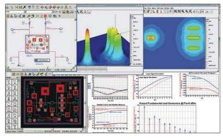
3. The ADS Electro-Thermal Simulator models and simulates temperature effects on RF/microwave ICs. (Photo courtesy of Keysight Technologies)
