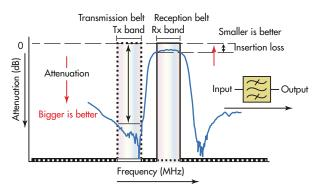
The use of BAW technology for wireless telecommunications has enabled higher Q filters at higher frequencies, and with lower form factors, than alternative filter technologies at similar frequencies.
