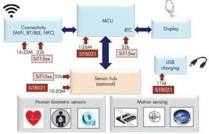
4. The lower-frequency model SiT1552 and 1-to-26-MHz model SiT8021 MEMS-based oscillators can serve a wide range of wearable, IoT, and mobile electronic products.
