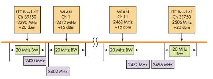
Many wireless portable devices contain both Wi-Fi and cellular hardware that may lead to Wi-Fi receiver desensitization if operating simultaneously.
