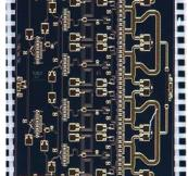
2. Model CMPA1D1E030D is a GaN MMIC amplifier chip on a SiC substrate capable of 30 W output power from 13.5 to 14.5 GHz.
