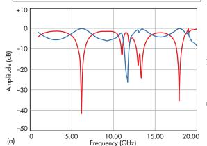
These plots show (a) S-parameters and (b) equivalent permeability for a Z-type metamaterial unit.
