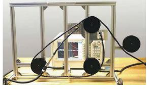
Gore's Cable Installation Simulator replicates the conditions a cable assembly experiences while being routed during installation in an aircraft. (Image courtesy of W.L. Gore & Associates)
