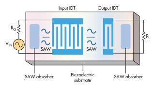
SAW filters employ interdigital transducers to create mechanical acoustic waves from electrical signals.
