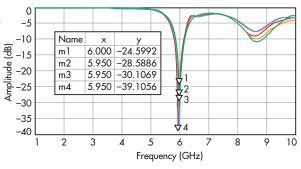
7. This is a plot of the return loss for the antenna design.
