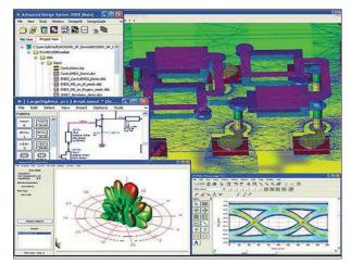
1. The Advanced Design System (ADS) software can model everything from devices through complete systems, using reasonable computer requirements. (Photo courtesy of Keysight Technologies)
