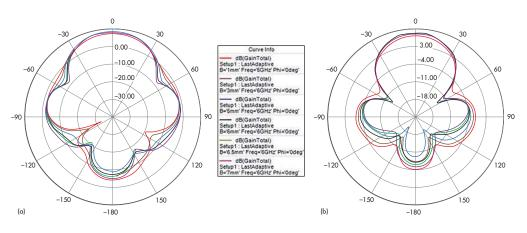
12. The distance between the covering layers and the antenna affects gain in (a) the E plane and (b) in the H plane.
