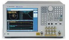
2. The E5072A ENA Series of vector network analyzers combine PIM testing with S-parameter measurements through 8.5 GHz. (Photo courtesy of Keysight Technologies)
