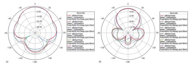
10. These plots show how the distance between cover layers and the antenna impacts gain in (a) the E plane and (b) in the H plane.
