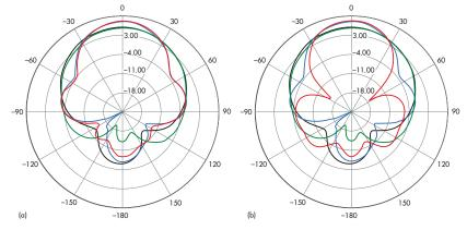
8. These plots show the gain of the antenna design in (a) the E plane and (b) in the H plane.
