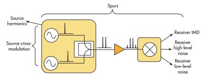
4. The third-order intercept is a measure of the depth of distortion created by intermodulation products.
