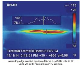
4. As this thermal display for a 50-W filter shows, RT/duroid 6035HTC material promises reliable PTHs even at the power/temperature levels of microwave PAs.
