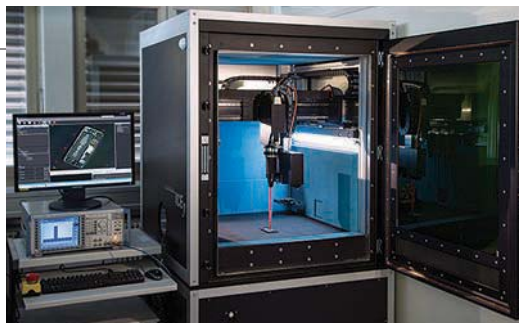
3. Using a machine-vision feedback network can increase the resolution of 3D positioning. (Courtesy of Speag)
