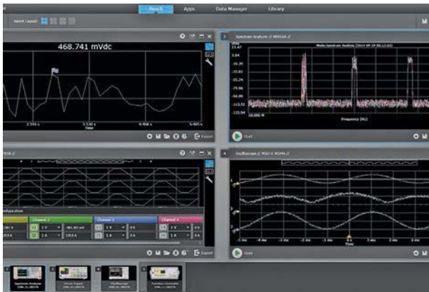
1. Using the measurement view, BenchVue can be used to correlate results from different measurements in one PC.
