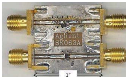
3. All the candidate solutions are evaluated using this common PCB test platform.
