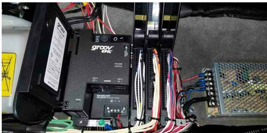
The groov EPIC embedded inside the truck's lift system.
