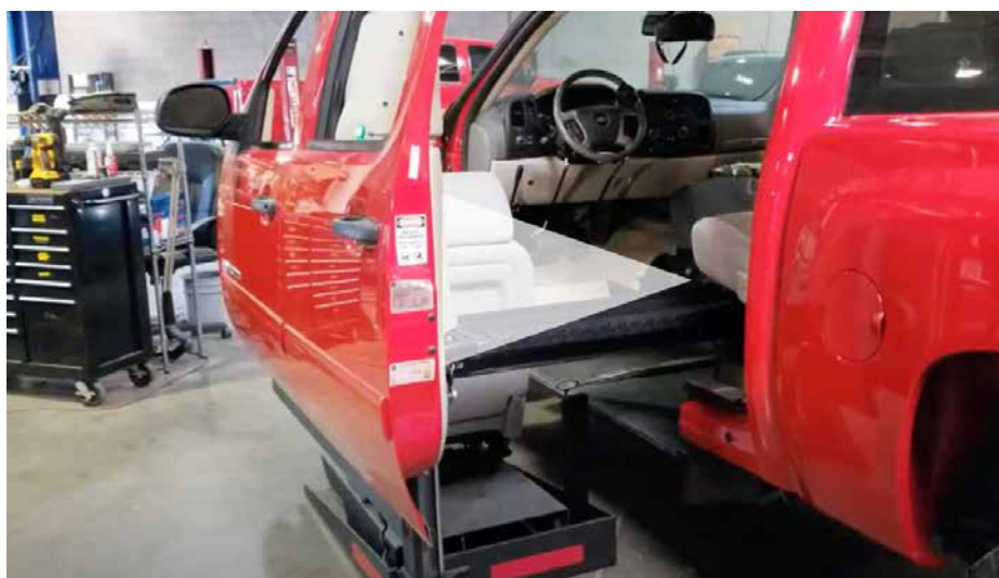
Take a look at DM's Silverado upgrade in this video, showing a full deploy-stow time under 30 seconds.
