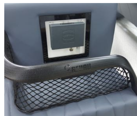
IIC MICA is being installed in Rinspeed's "Etos" concept car for independent emissions and status monitoring.
