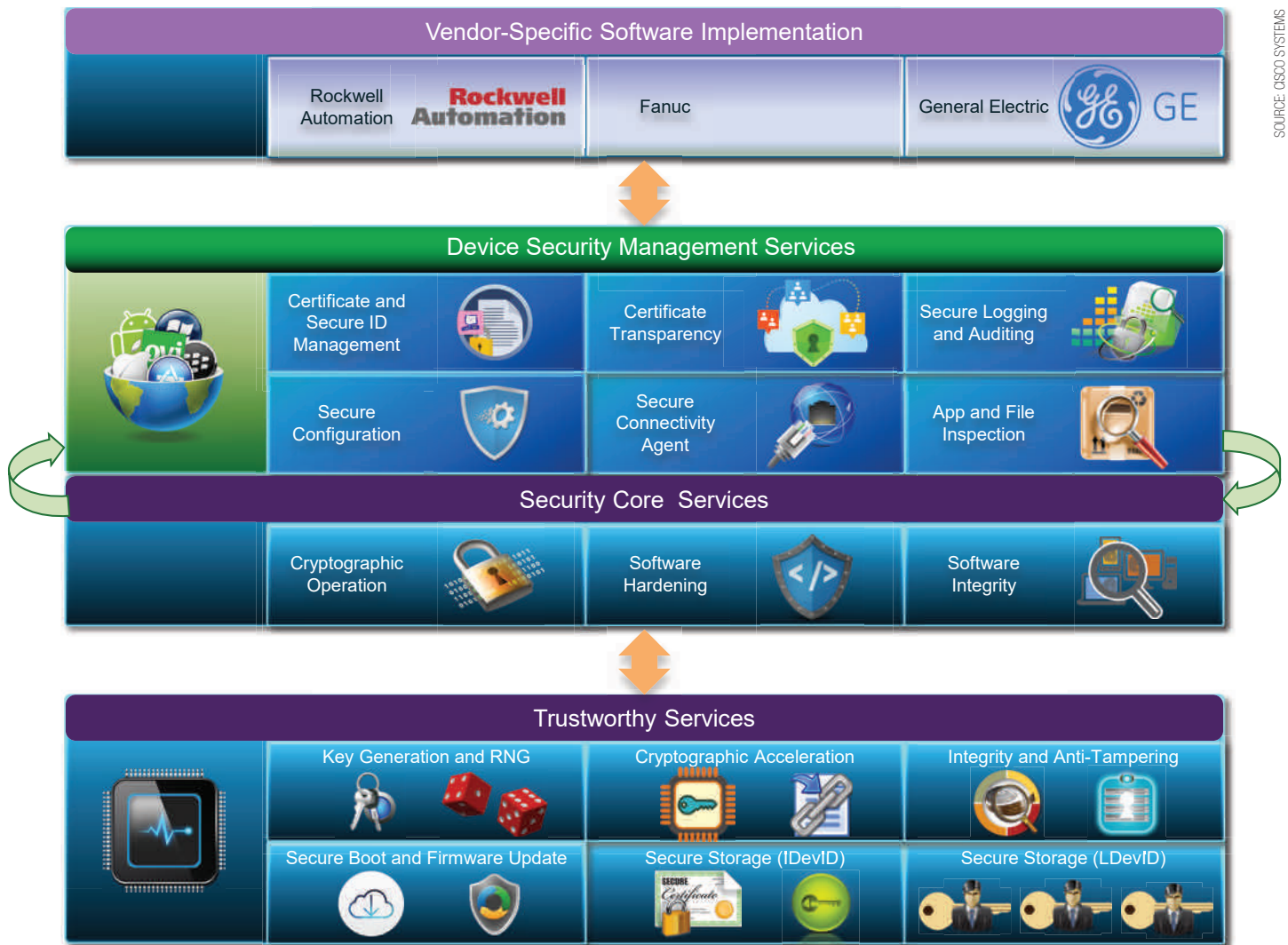
Reference Architecture of Trustworthy Device. With a general framework and components defined, different levels of security and trustworthiness can be achieved.
