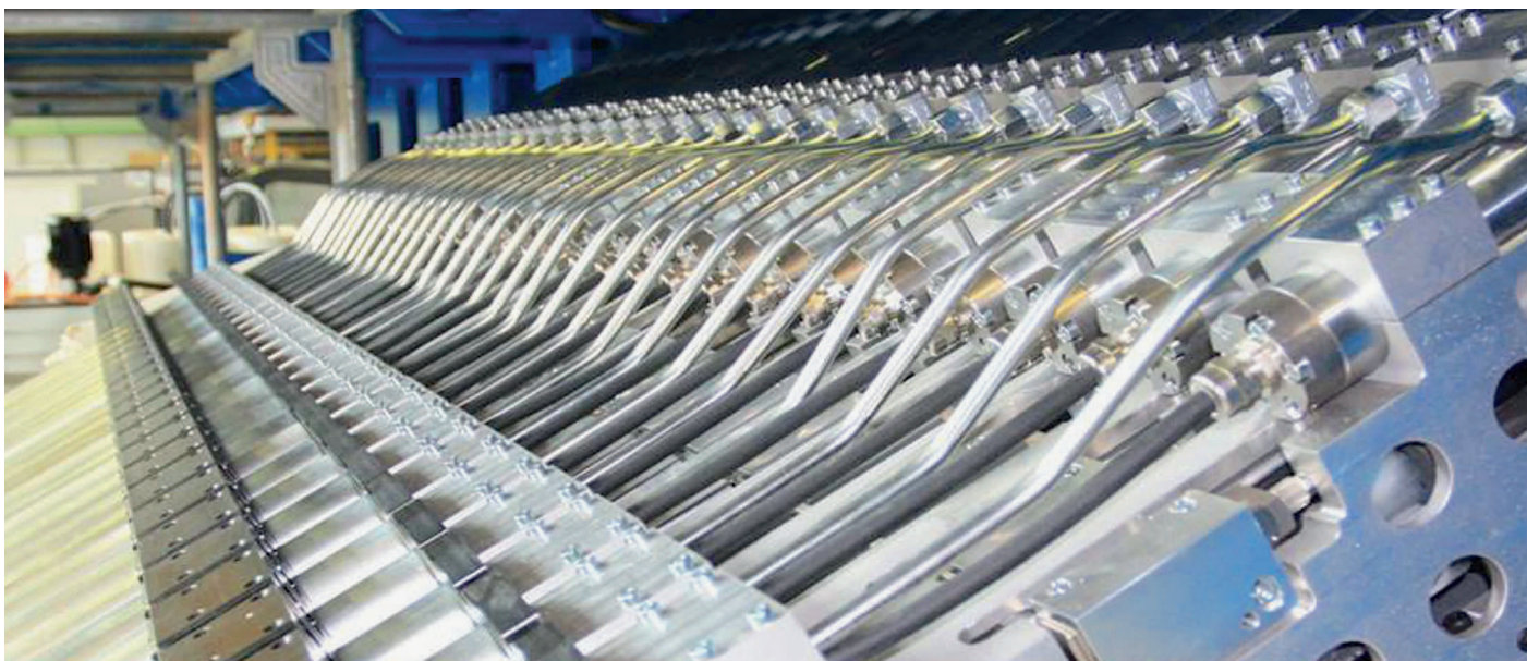
Nonferrous linear motors move 60 electrodes with great precision, leveraging the speed of the high speed Sercos motion network.
