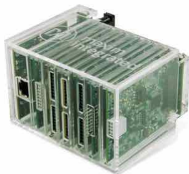
One way to supporting Industry 4 Micro PLC Reference Design shows how much space can be saved when engineers take advantage of new analog integration.
