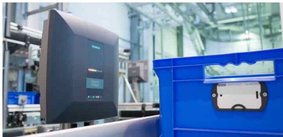
New RFID readers with adaptive antennas are easy to configure for different environmental conditions.
