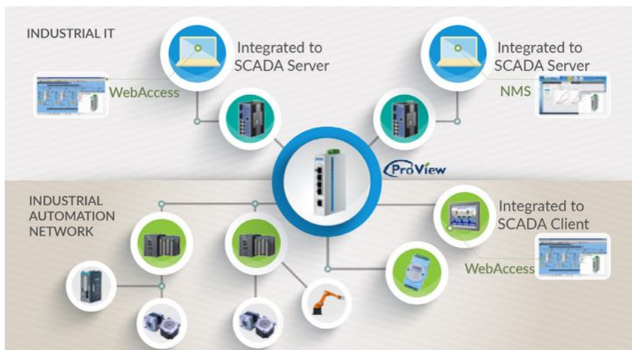
To allow automation and IT software to monitor status, the switch technology supports both Modbus/TCP and SNMP.
