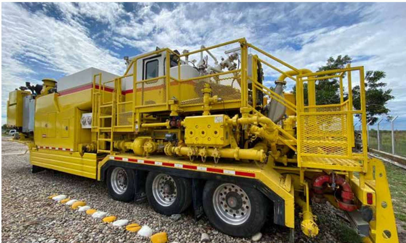
Tucker Energy Services well cementing unit.
