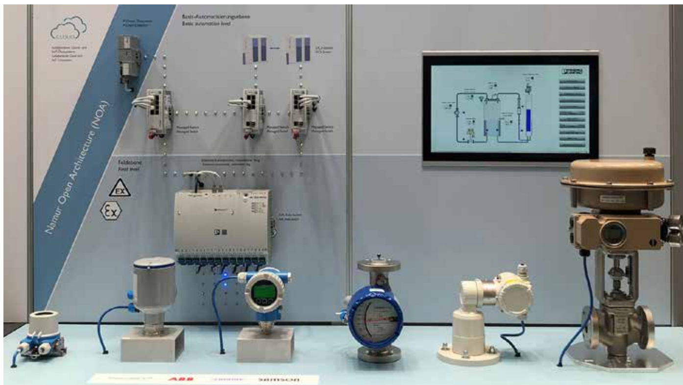
Figure 1: The first public demo with APL was presented at the NAMUR Congress in November 2019. Together with Endress+Hauser, KROHNE, ABB and SAMSON, the field switch accentuated the capabilities of the intrinsically safe APL field devices. Other Phoenix Contact products used in the scope of delivery for APL projects include managed Ethernet switches, cybersecurity, monitoring and optimization systems, power supplies, Fieldbus and process I/O solutions. (Photo taken in August 2022 at AICHEMA and fully functional).
