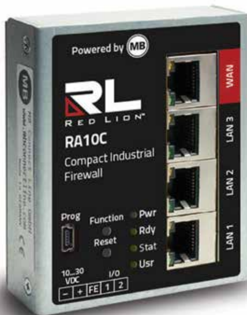
Red Lion's RA10C compact industrial firewall
