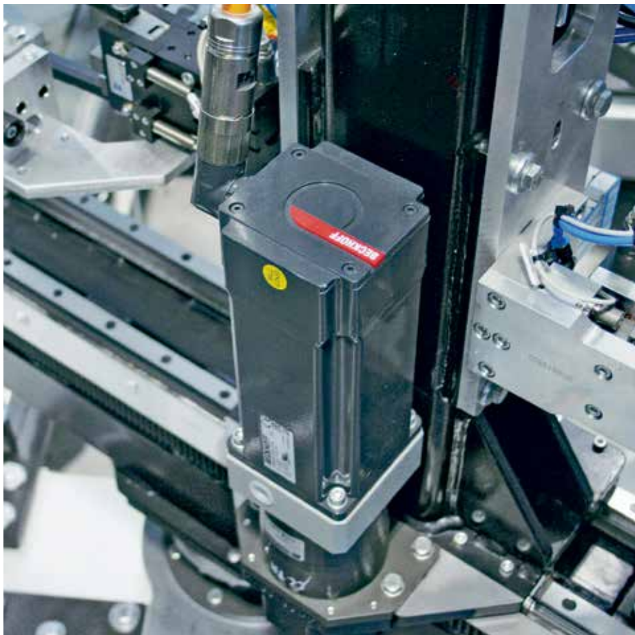
The distributed connection concept based on EtherCAT P and the compact AMP8000 servo drives save valuable space in the machine.
