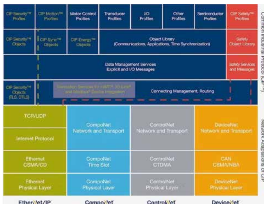
Figure 4. EtherNet/IP as per the typical OSI Layer
