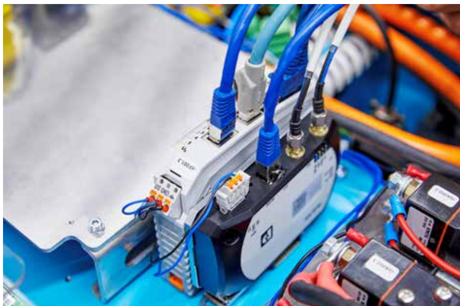
The FL WLAN 1010 wireless module in the AGV, mounted directly on the vehicle chassis or a DIN rail, has two antenna inputs for improved wireless quality.
