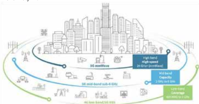
Figure 2.a 5G mmWave spectrum. Figure 2.b Typical use cases of 5G in smart manufacturing.
