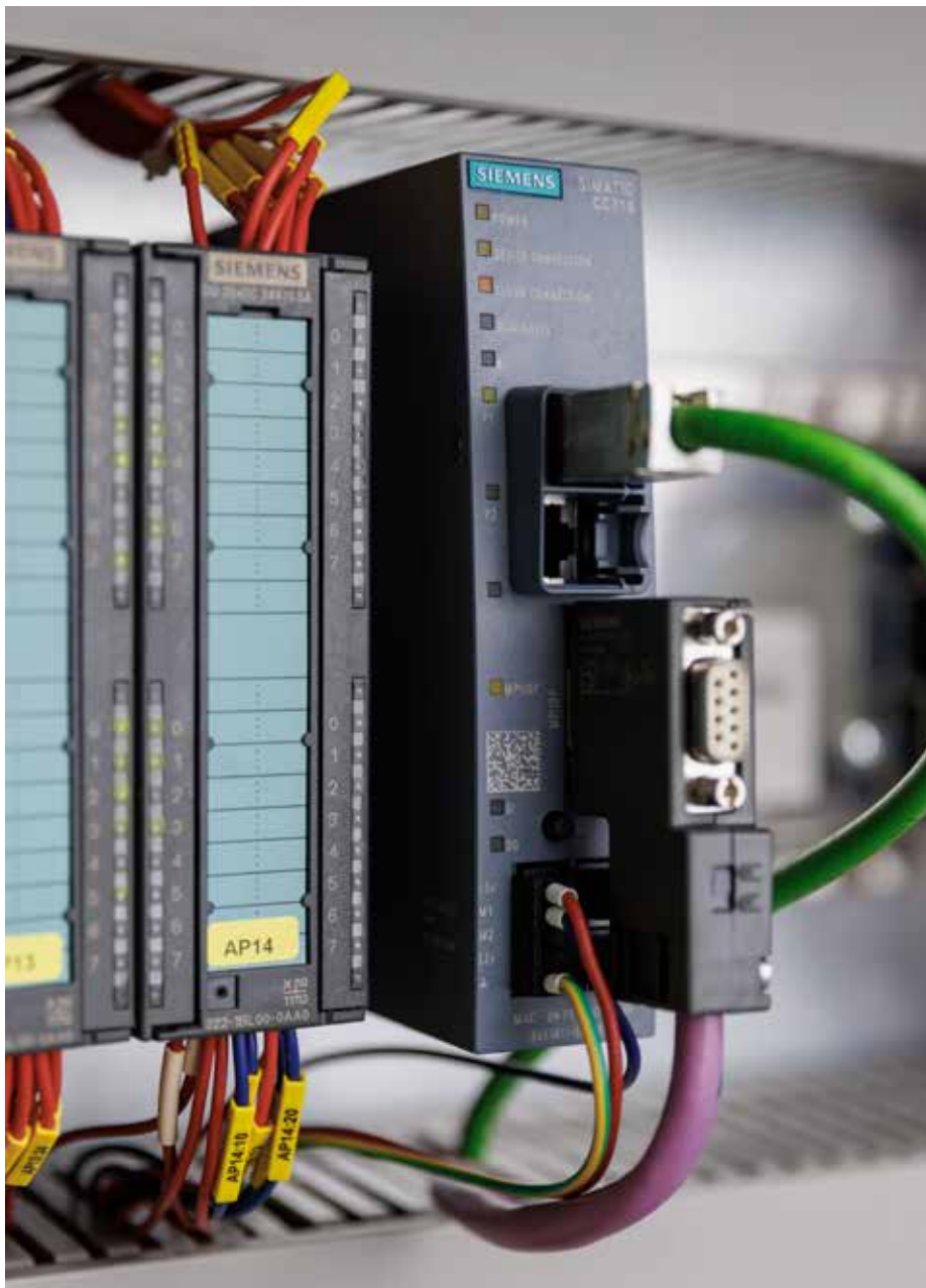
The Simatic CC716 industrial IoT gateway supports connection via Industrial Ethernet or the Profibus/MPI interface.
