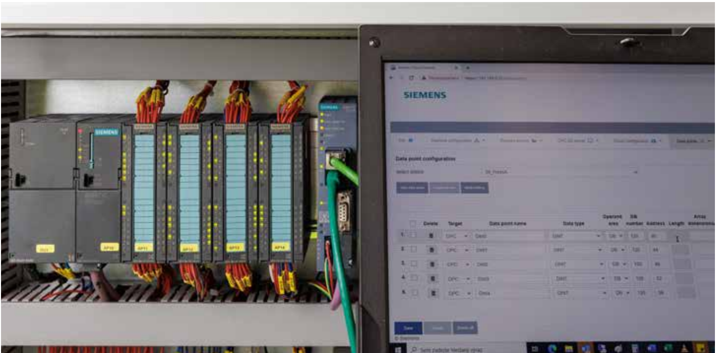
Convenient configuration of data points (from PLC to an OPC UA server) via a Simatic CC716 web server module with no need to change hardware configuration in Step 7.
