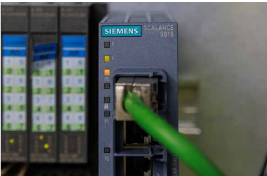
The Scalance S615 NAT router converts data from the internal network to the external network.
