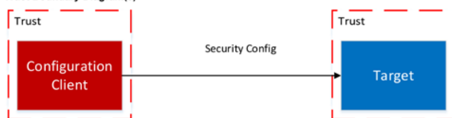
Figure 1: Trust boundary and data flow for CIP Security Push Model.
