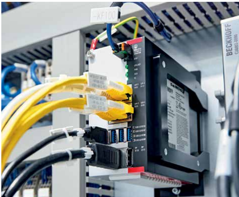
A C6030 ultra-compact Industrial PC provides optimal computing power for central control of all process sequences.
