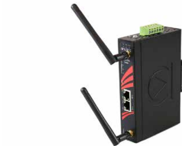
ARS-7235-PSE-AC is an industrial-hardened dual-radio IEEE 802.11a/b/g/n/ac wireless LAN access point.
