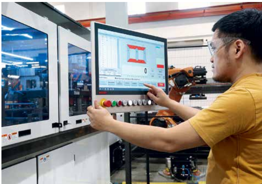
The 21.5-inch CP3921 multi-touch Control Panel with custom push-button extensions provides operator interface for the cutting cell, with a smaller touchscreen on the stacking cell.
