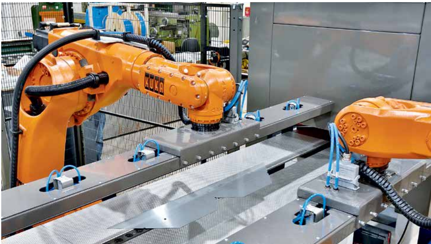
The two articulated KUKA robots stacking the cut laminations can be integrated optimally with PC-based control technology from Beckhoff.
