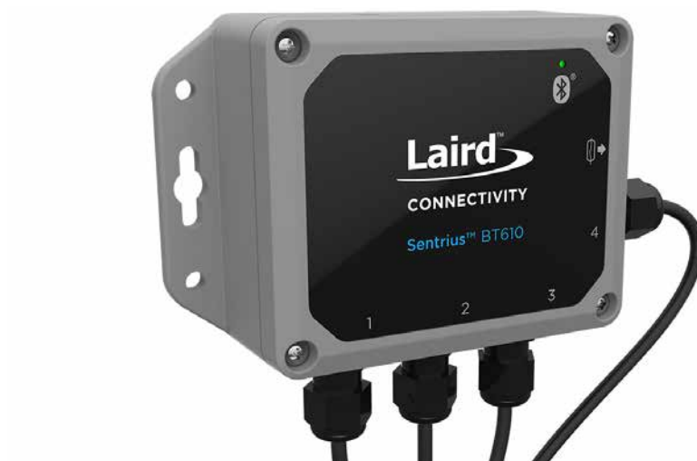
The BT610 supports virtually any industry-standard external sensor through a wide range of interface options.
