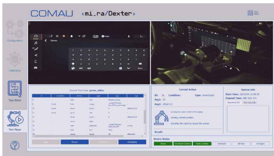
Programming interface enables operators to adjust and correct the actions of the robot in real-time.
