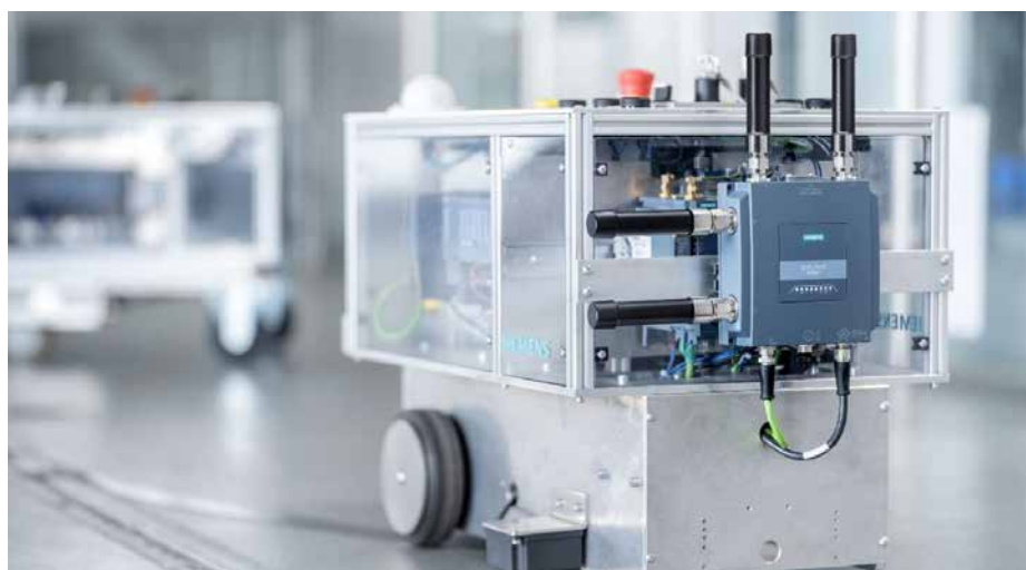
The Scalance MUM856-1 supports Release 15 of the 5G standard.
