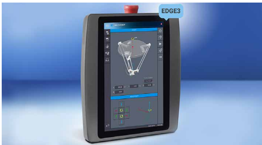
The 10.1" HGT 1053 mobile panel offers a multi-touch screen, high visualization power and safety elements.
