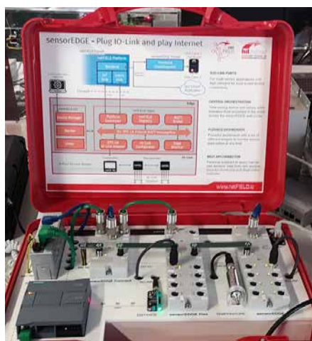
The demo box for the sensorEDGE gateways illustrates there is no need for a PLC or IO-Link Master to connect sensor data to the internet.
