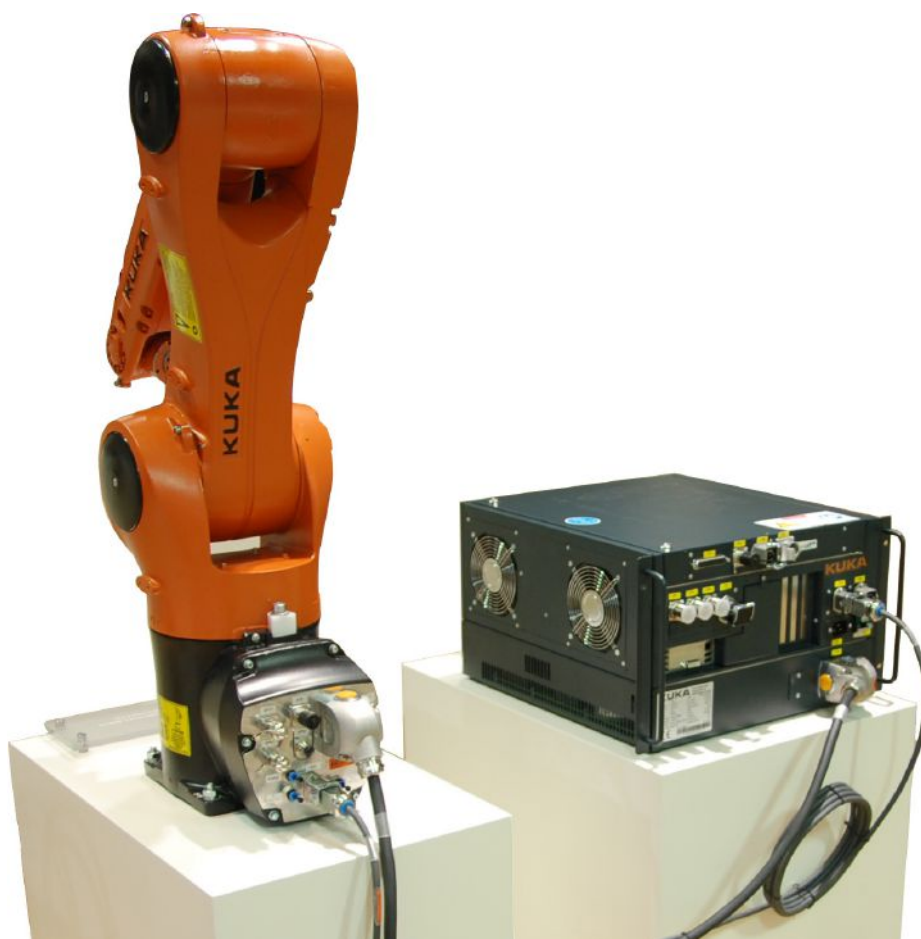
Han-Yellock connector system on KR AGILUS robot system from KUKA.
