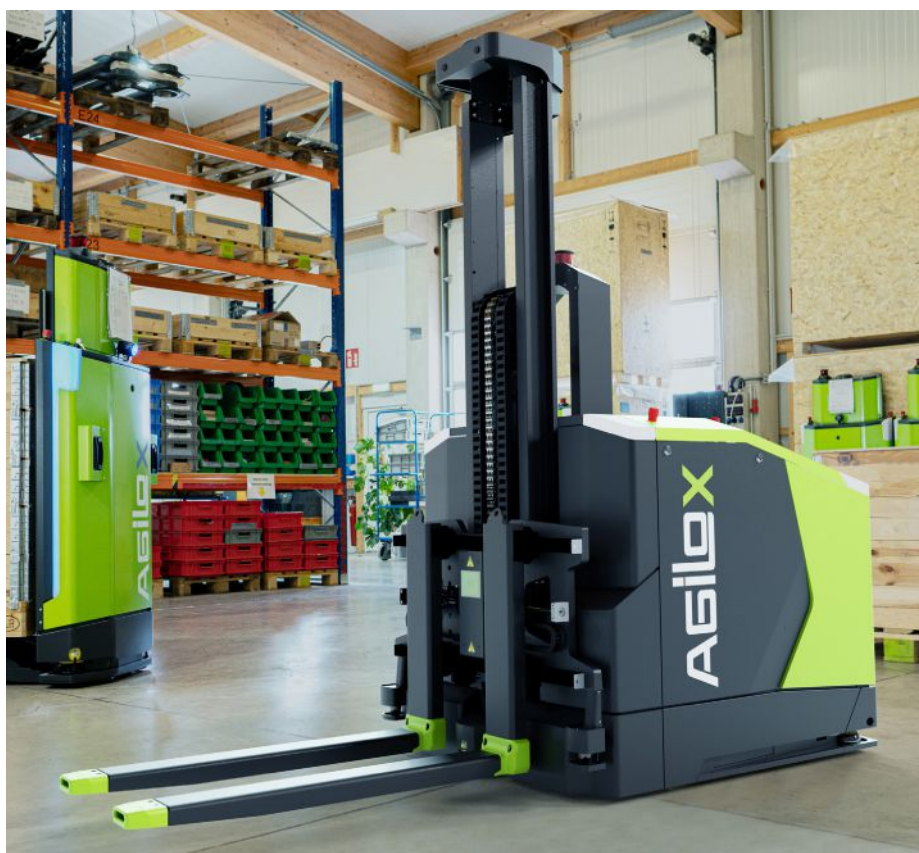
Autonomous counterbalanced forklift navigates factory by using swarm intelligence.
