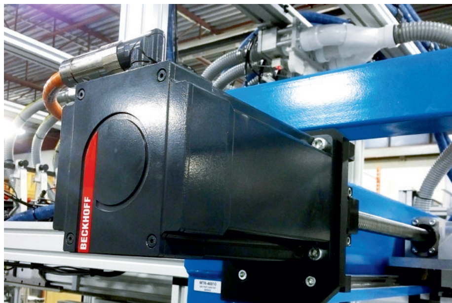
The AM8000 series servomotors with OCT handle conveyance, pick and place, web lamination, tension control and height adjustments.
