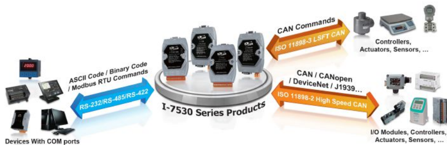
Transparent communication functionality adds CAN communication functions to traditional UART devices.
