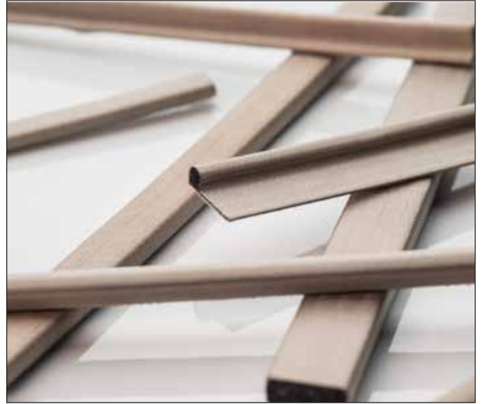
Figure 5 • Metalized fabric gaskets from are manufactured with a polyurethane foam core and nickel-plated copper-conductive fabric.
