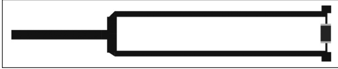
Figure 2 • Layout of a microstrip Wilkinson Power Divider (top layer) with a chip resistor.
