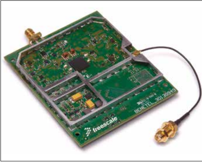
Figure 6 • The femtocell reference platform based on Freescale's baseband architecture and RF devices, built by Benetel, and available to designers.
