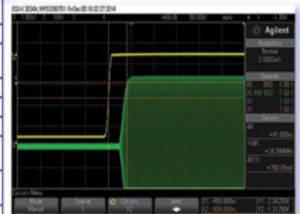
Sideband Switching Speed 45ns Measured
