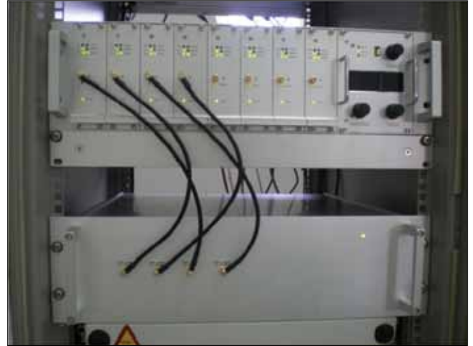
Figure 7. Front view of the IF processor (bottom rack) installed in the backend room below the FFTS.
