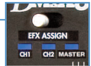
Fig 8.7 Channel assign switch
